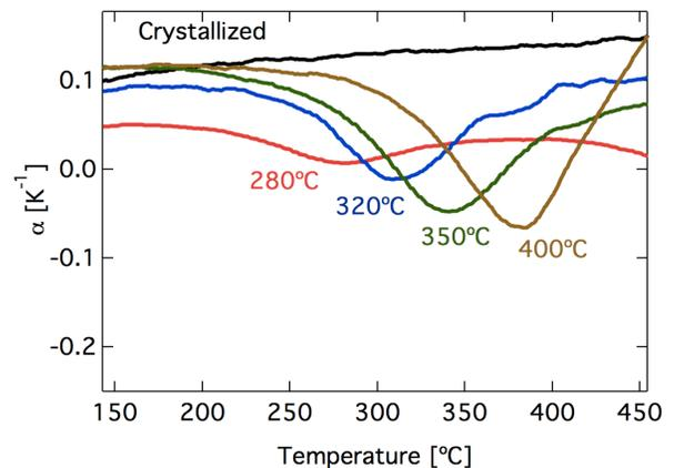
Fig. 1 Temperature dependence of LTE coefficient,  $\alpha$ , of amorphous  $\text{Co}_{72.5}\text{Fe}_{1.5}\text{Mn}_4\text{Si}_5\text{B}_{17}$  ribbons with the different annealing temp. indicated in the graph.
