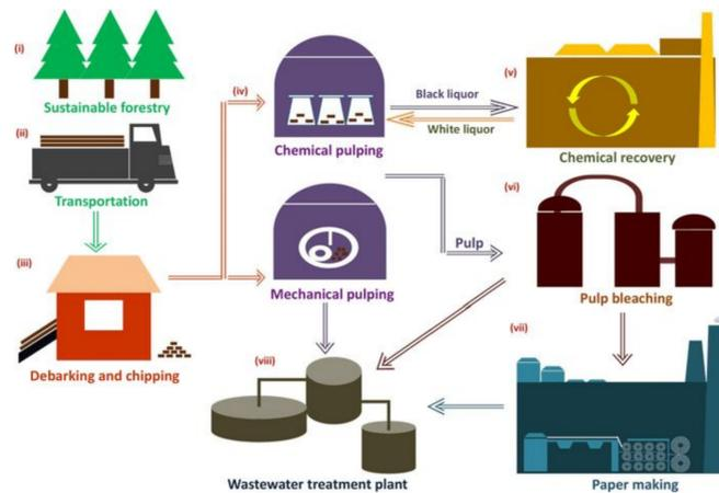
Figure 1: Paper manufacturing process
