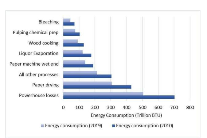
Figure 4: Energy consumption by process (2019)<sup>2</sup>
