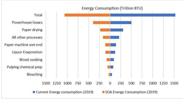
Figure 5: Comparison of energy consumption between current and SOA (2019)<sup>2</sup>
