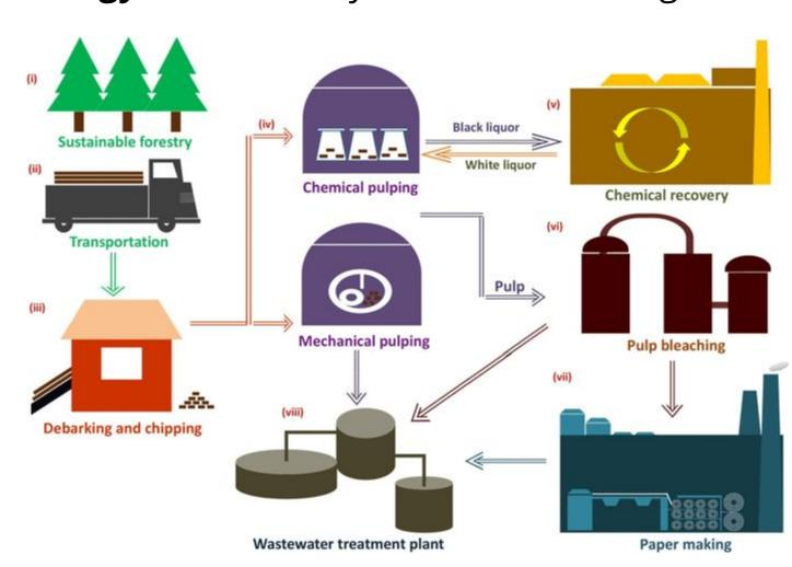
Figure 1: Paper manufacturing process
