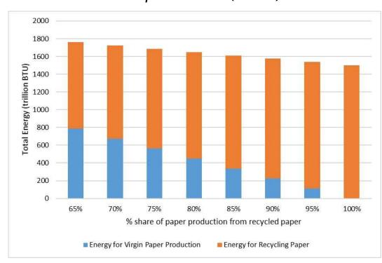
of paper produced, replacing wood with used paper as raw material entirely has the potential to reduce total energy demand by 15% as compared to the existing scenario (65% used paper).
