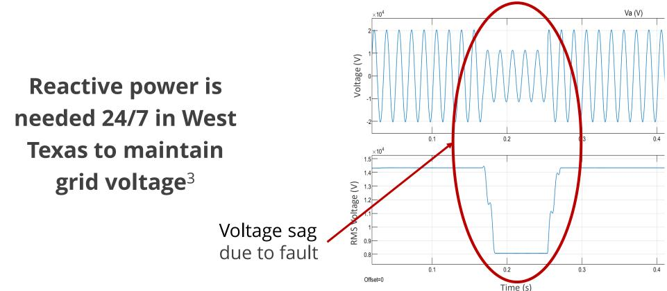
During the day, when the sun is shining PV plants can produce and consume reactive power to support voltage on the grid. At night, this support disappears, and the PV plants no longer provide that reactive power for voltage support. This has led to the installation of two expensive STATCOMs in West Texas in 2018, costing \$70 million<sup>3</sup>.
