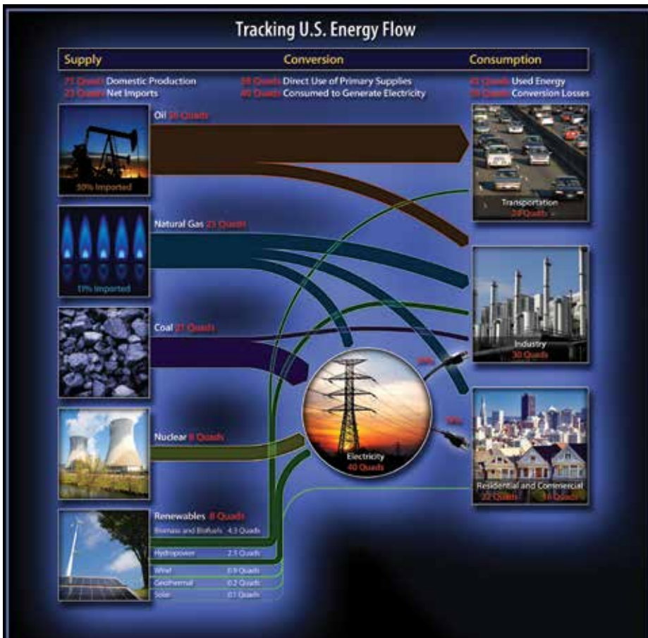
Figure 1: Energy Generation and Consumption Flows, 2010. This diagram shows 2010 energy flow from primary sources (oil, natural gas, coal, nuclear, and renewables) through transformations (electricity generation) to end uses (transportation, industry, and residential, and commercial sectors). Oil provided the largest share of the 98 quads of primary energy consumed, and most of it was used for transportation. Consumption of natural gas, the nation’s second largest energy source, is split three ways—electricity generation, industrial processing, and residential and commercial uses (mostly for heating). Coal, our third largest source, is used almost exclusively for electricity. Nuclear energy and renewables each meet less than 10% of U.S. energy demand.
