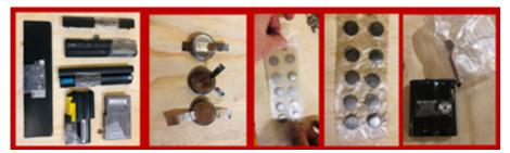
Batteries taped for recycling
