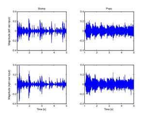
Figure 8: Waveform comparison between binaural signals for "Stomp" and "Pops." The two panels on the left show the waveforms for "Stomp" while the panels on the right show "Pops." The top row shows the left-ear signal and the bottom row shows the right-ear signal.
