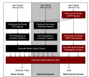
Figure 6: One example approach for extending ITU-R BS.1387-1 to multi-channel use.
