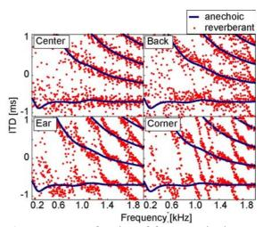
**Fig. 5** ITDs as a function of frequency in the anechoic and reverberant conditions for source at 90° 1 m.
