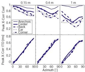
**Fig. 4** The peak value in the cross-correlation function within +/- 1 ms range and the corresponding ITD.
