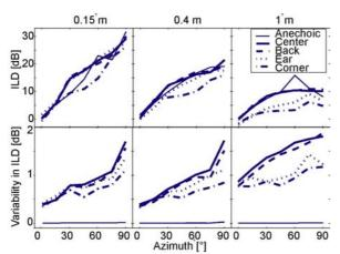
**Fig. 3** ILDs and cross-frequency variability in ILDs at 4 room locations as a function of source azimuth.
