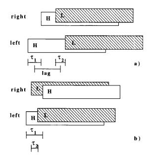
FIG. 1. Schematic diagram of stimuli. Binaural noise bursts with either high- (H) or low- (L) frequency content were presented with interaural time delays  $\tau_1$  and  $\tau_2$ , with a delay (called lag) between mean onsets. (a) Diagram showing bursts when lag is 1 ms (experiments 1 and 3). (b) Diagram showing bursts when lag is 0 ms (experiment 2). In this case,  $t_2$  refers to the interaural delay in the L stimulus.
