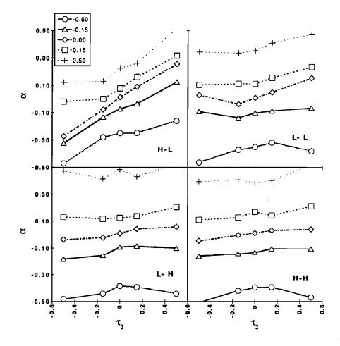
FIG. 2. Interaural delay of the pointer ( $\alpha$ ) as a function of  $\tau_2$ , the interaural delay of the lagging burst in the test stimuli. The interaural delay of the leading burst ( $\tau_1$ ) is shown parametrically. Each panel shows results for one of the four frequency conditions averaged across subjects.
