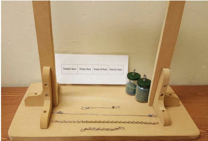
FIGURE 3. Pendulum materials for Study 2, with four strings of two lengths and two materials plus two jars of different weights.
