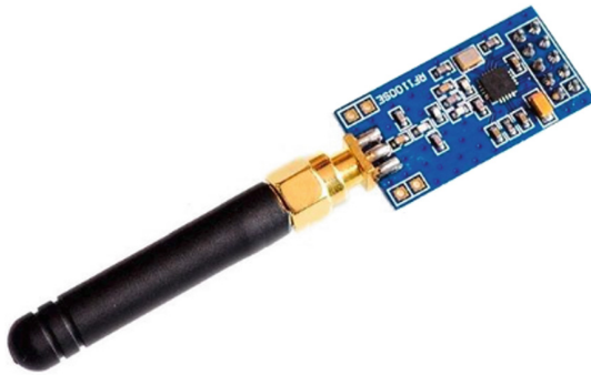
Fig. 6. CC1101 module used in our prototype for validation
