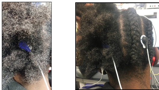
Fig. 3. Traditional EEG gel based EEG methods do not work satisfactorily with different hair types ( left ). Modification of hair structure can provide reliable methods of obtaining stable EEG measurements.
