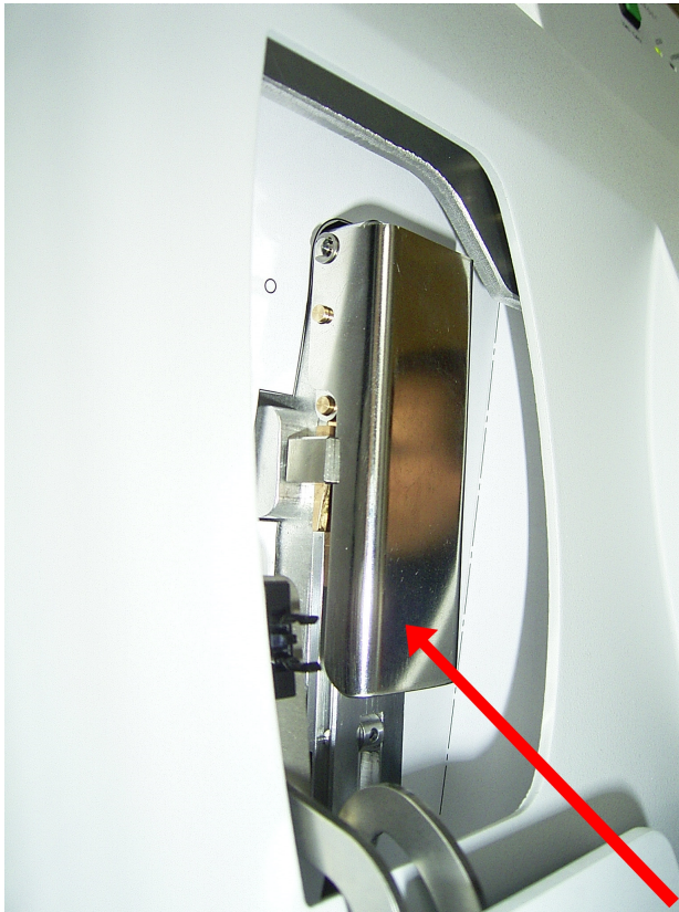
Figure 5-3 Opening the cover plate of the manual cartridge
