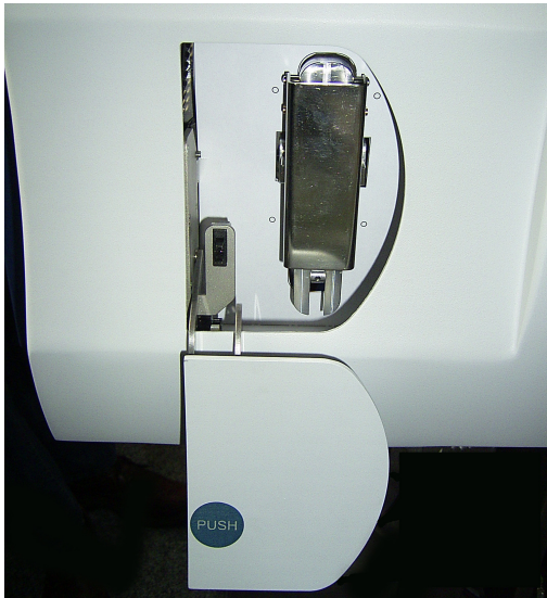
Figure 5-2 Open cover lid giving free access to the manual cartridge
