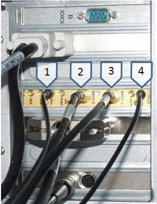
Figure 2-2 Connections at the rear of the PC 1 Digitizer Sync (Handshake), MCX connector 2 Input 2 – Reflector, SMA connector 3 Input 1 – Linear, SMA connector 4 Trigger, MCX connector
