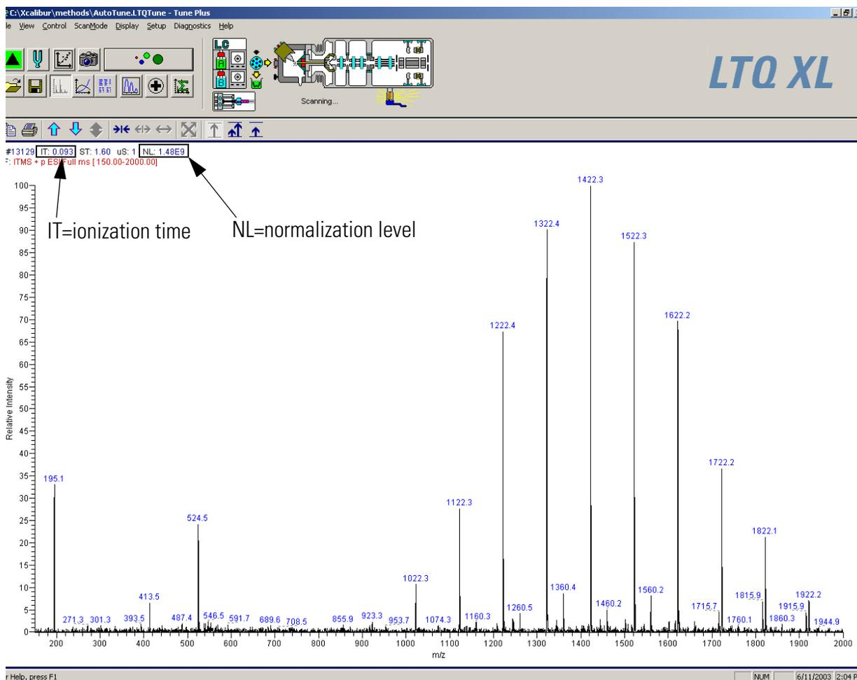
Figure 22. Spectrum view of the Tune Plus window, showing ionization time (IT) and normalization level (NL) of the calibration solution
