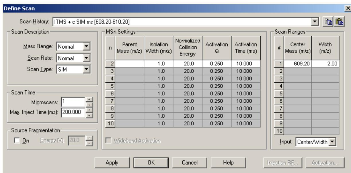
**Figure 59.** Define Scan dialog box, showing typical settings for APCI/MS operation
