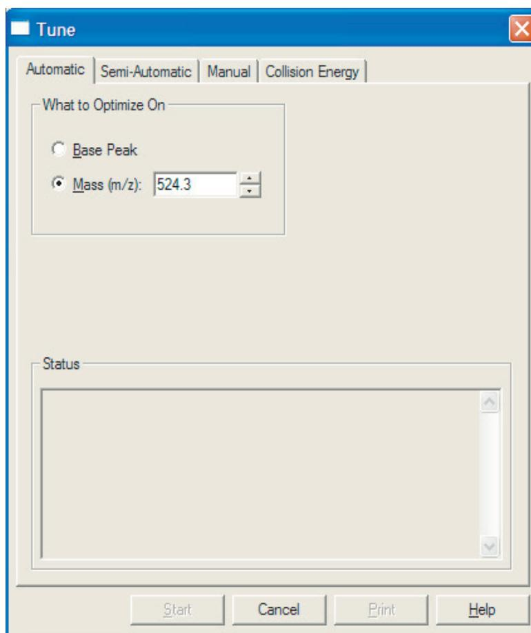
**Figure 71.** Tune window showing the MS detector Tune on  $m/z$  524.3u
