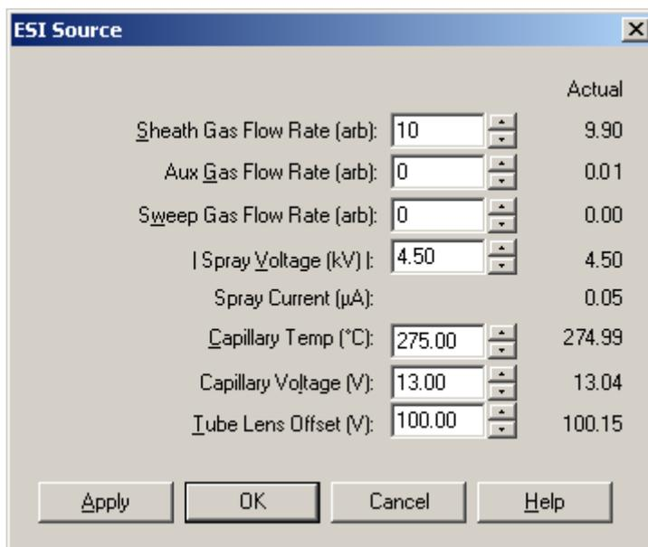
**Figure 19.** ESI Source dialog box, showing the settings to start a typical low flow experiment
