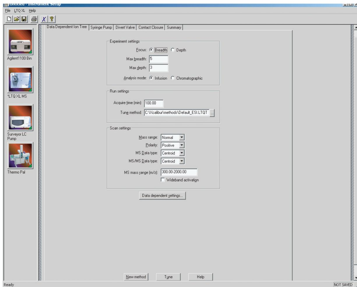
**Figure 4.** Data-Dependent Ion Tree page in Instrument Setup, showing a template for an Ion Tree experiment
