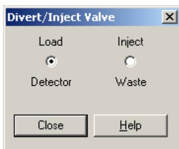
**Figure 68.** Divert/Inject Valve dialog box
