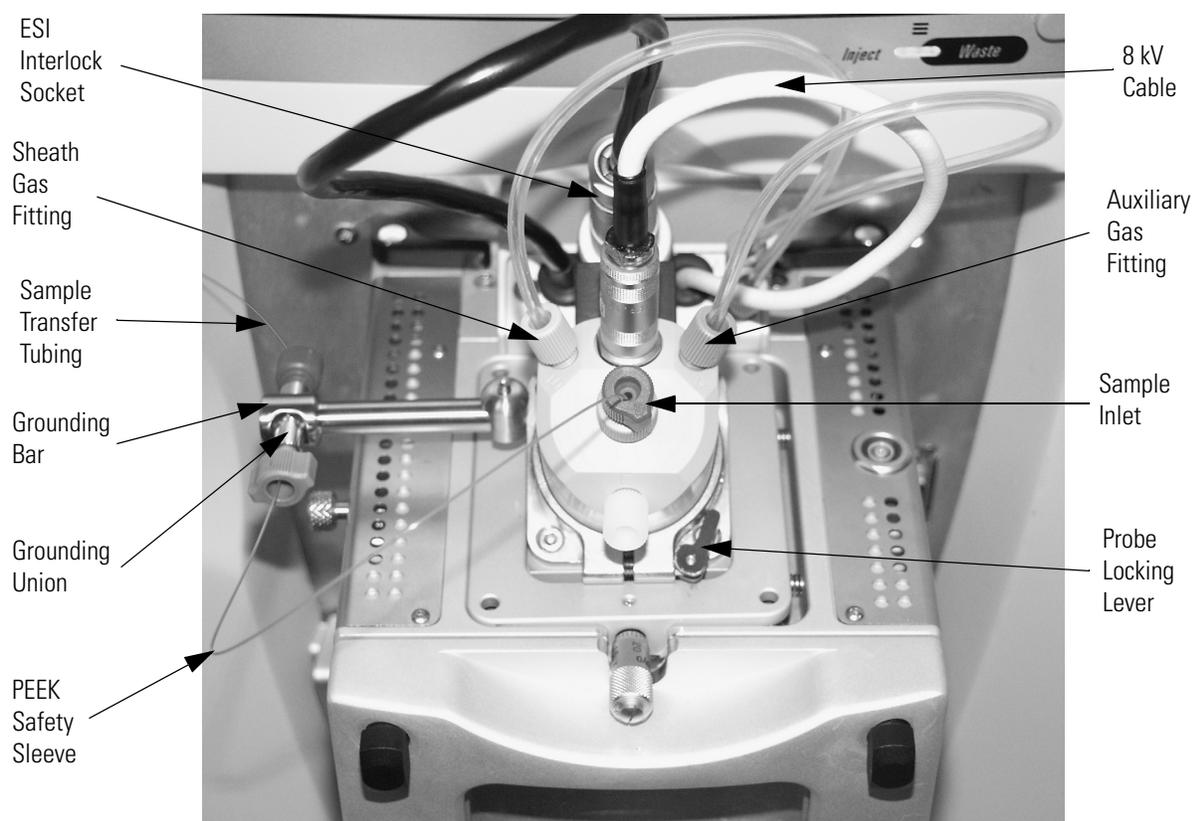
**Figure 50.** Ion Max ion source housing with ESI probe installed
