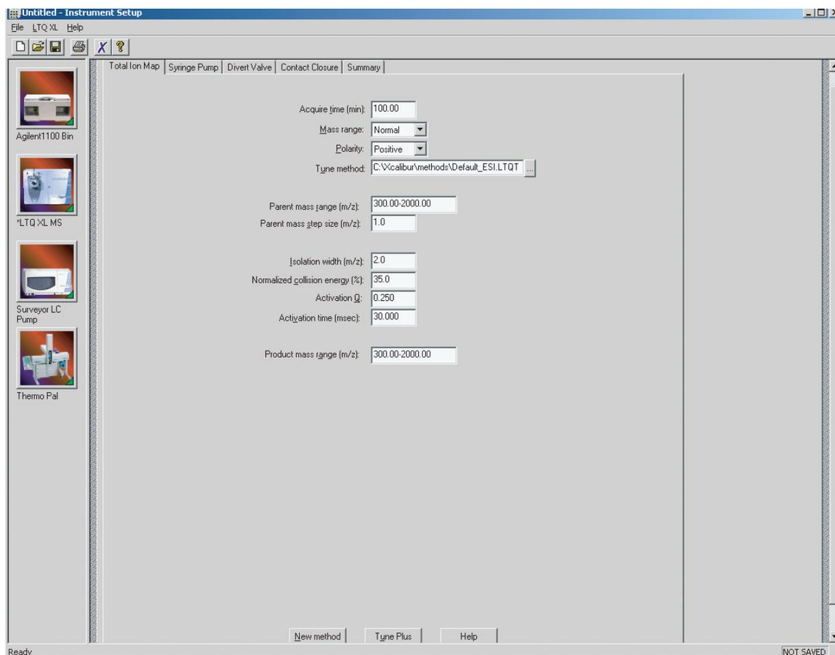
**Figure 3.** Total Ion Map page in Instrument Setup, showing a template that contains parameters for an Ion Mapping experiment
