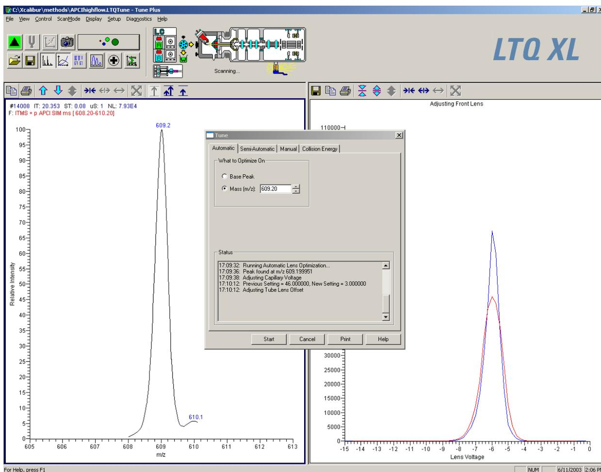
Figure 61. Tune Plus window with the Tune dialog box, showing the Automatic tuning page
