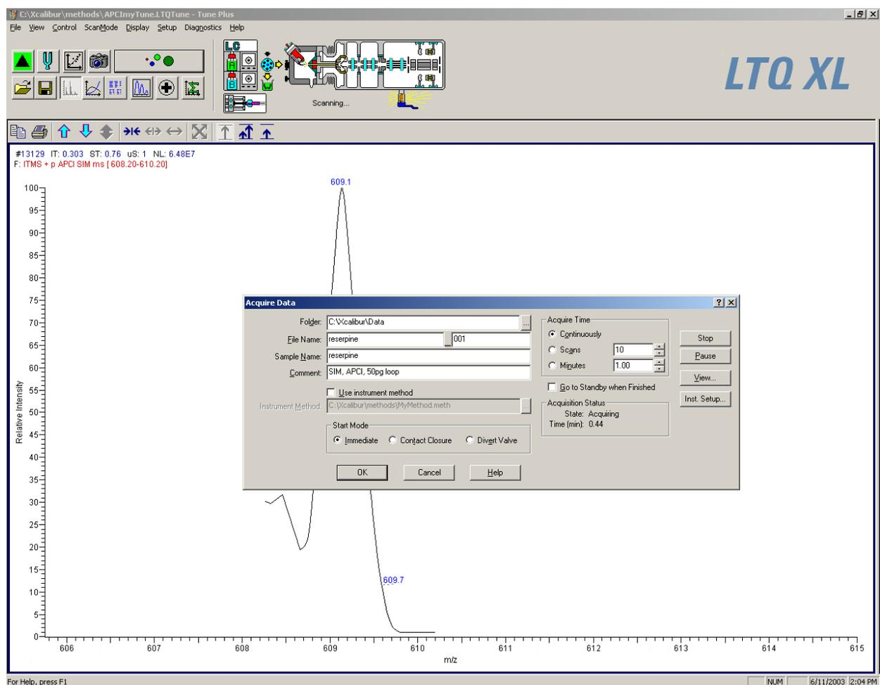
**Figure 67.** Tune Plus window, showing the SIM spectrum of reserpine during analysis by loop injection
