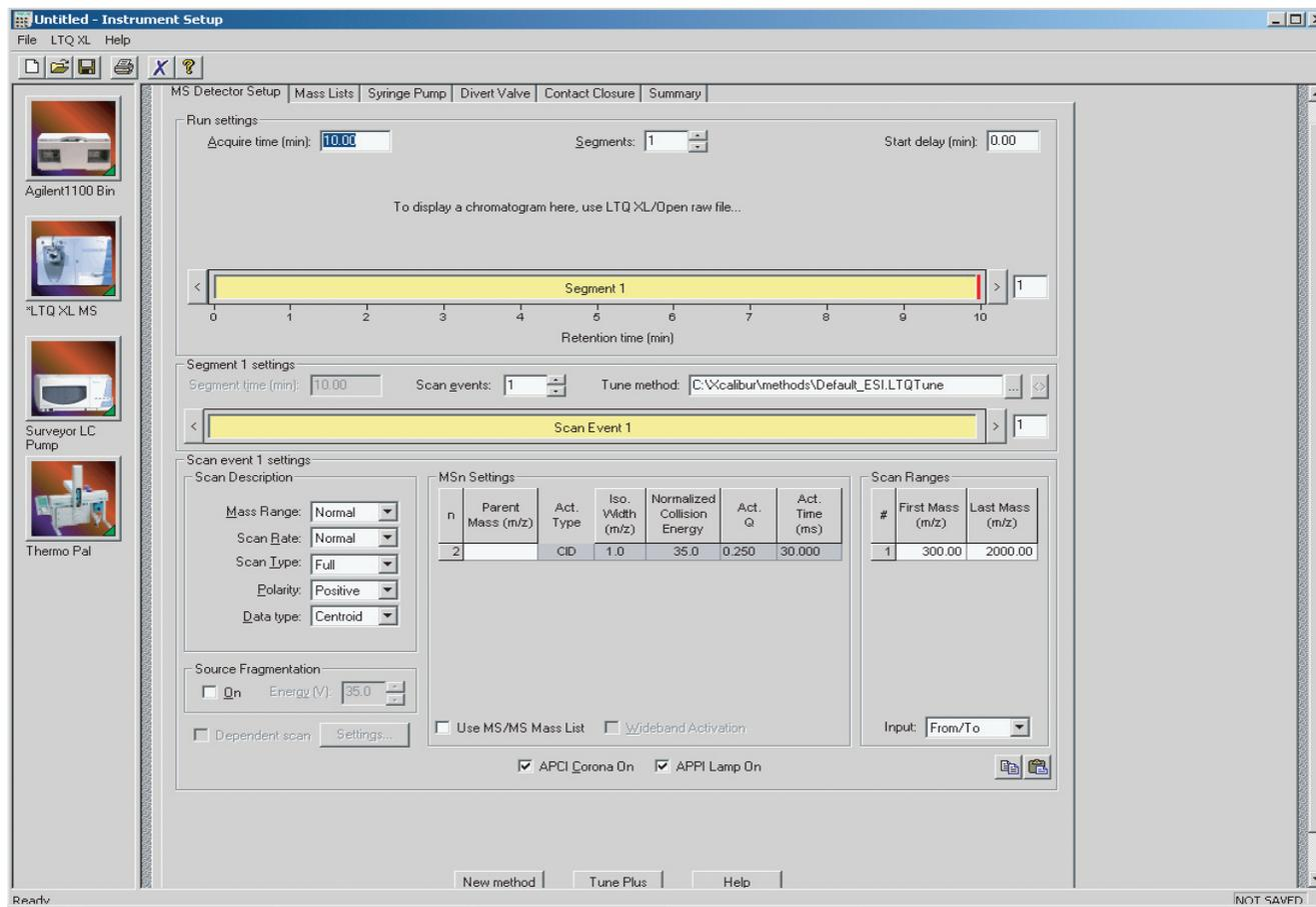
**Figure 1.** MS Detector Setup page in Instrument Setup, showing a template for a General MS experiment
