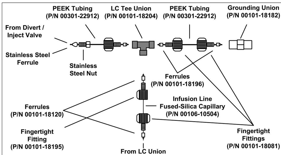
**Figure 57.** APCI/MS plumbing connections for the LC Tee union
