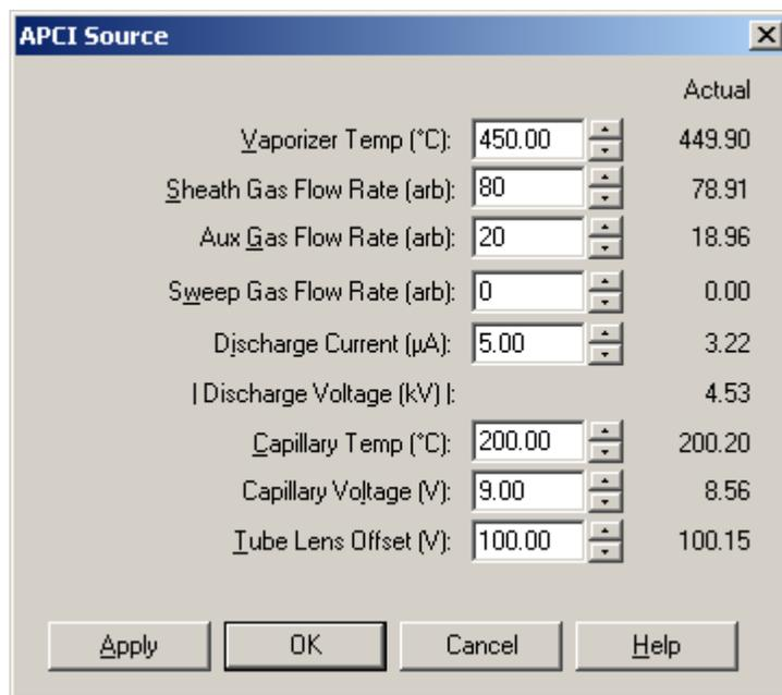
**Figure 58.** APCI Source dialog box, showing the proper settings for a typical high flow experiment
