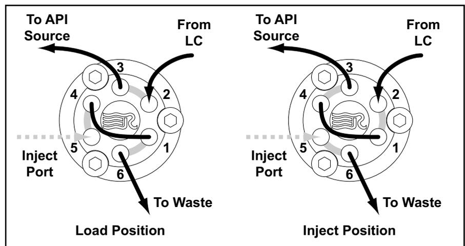
**Figure 63.** Divert/Inject valve, showing the correct setup for analysis by loop injection and showing the flow of liquid through the valve in the Load and Inject positions
