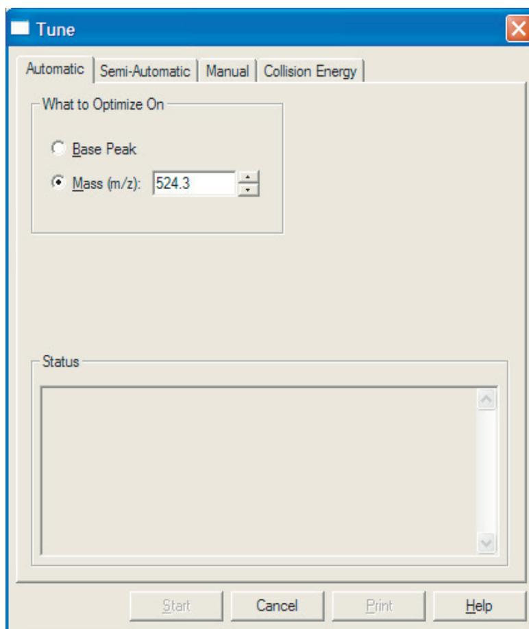
**Figure 71.** Tune window showing the MS detector Tune on  $m/z$  524.3u
