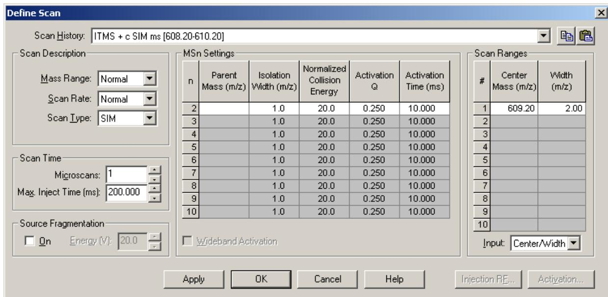
**Figure 45.** Define Scan dialog box, showing typical settings for acquiring reserpine data in the SIM scan type
