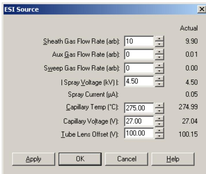
**Figure 25.** ESI Source dialog box, showing typical parameters after automatic tuning
