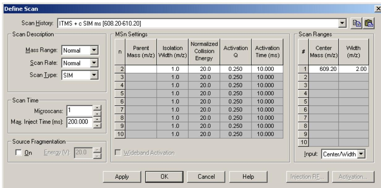
**Figure 32.** Define Scan dialog box, showing typical settings for acquiring reserpine data of the SIM type
