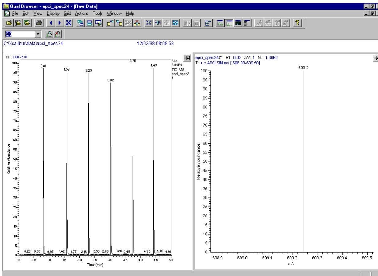
**Figure 69.** Qual Browser window, showing loop injections of reserpine in the Chromatogram view (left) and  $m/z$  609 in the Spectrum view
