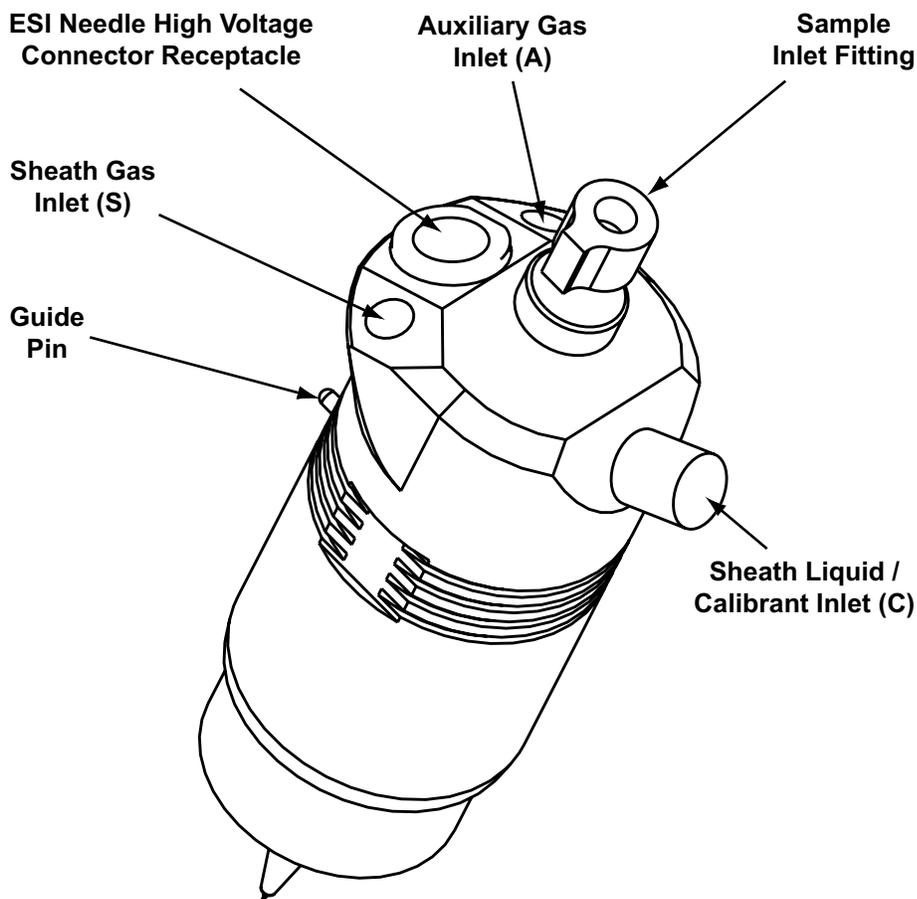
**Figure 14.** ESI probe, side view
