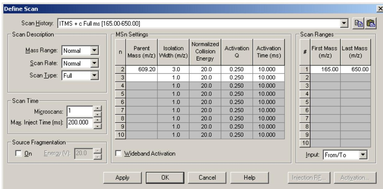
**Figure 37.** Define Scan dialog box, showing initial settings to optimize the isolation width of an MS/MS experiment for reserpine
