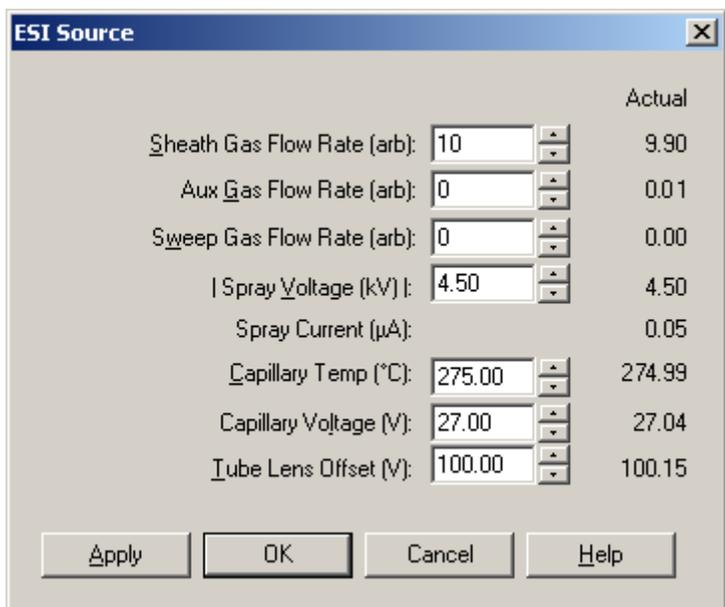
**Figure 25.** ESI Source dialog box, showing typical parameters after automatic tuning
