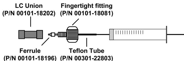
**Figure 16.** Plumbing connections for the syringe
