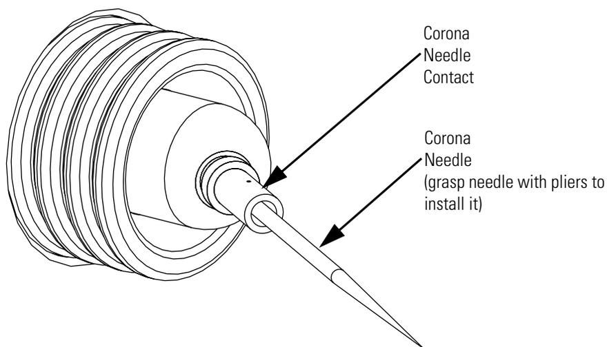
**Figure 52.** Corona needle, view from inside of the Ion Max housing
