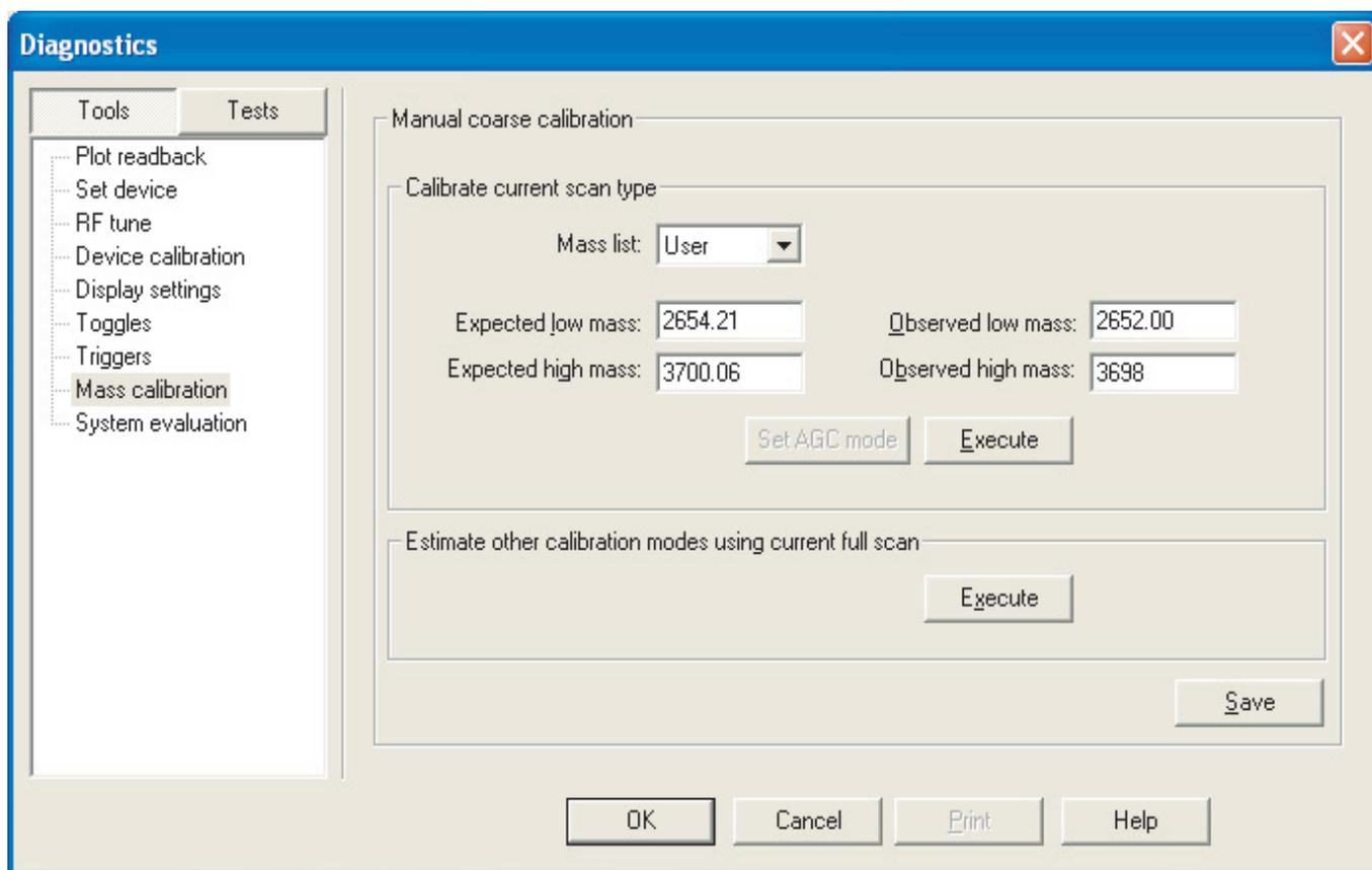
**Figure 73.** Tune Plus Diagnostics dialog box, two point high mass calibration
