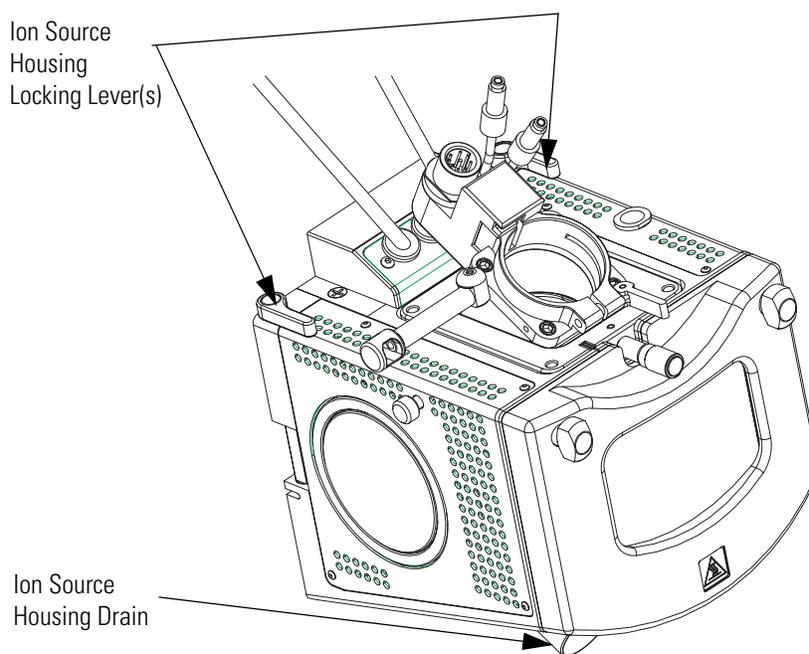
**Figure 51.** Ion Max ion source housing, detail of components
