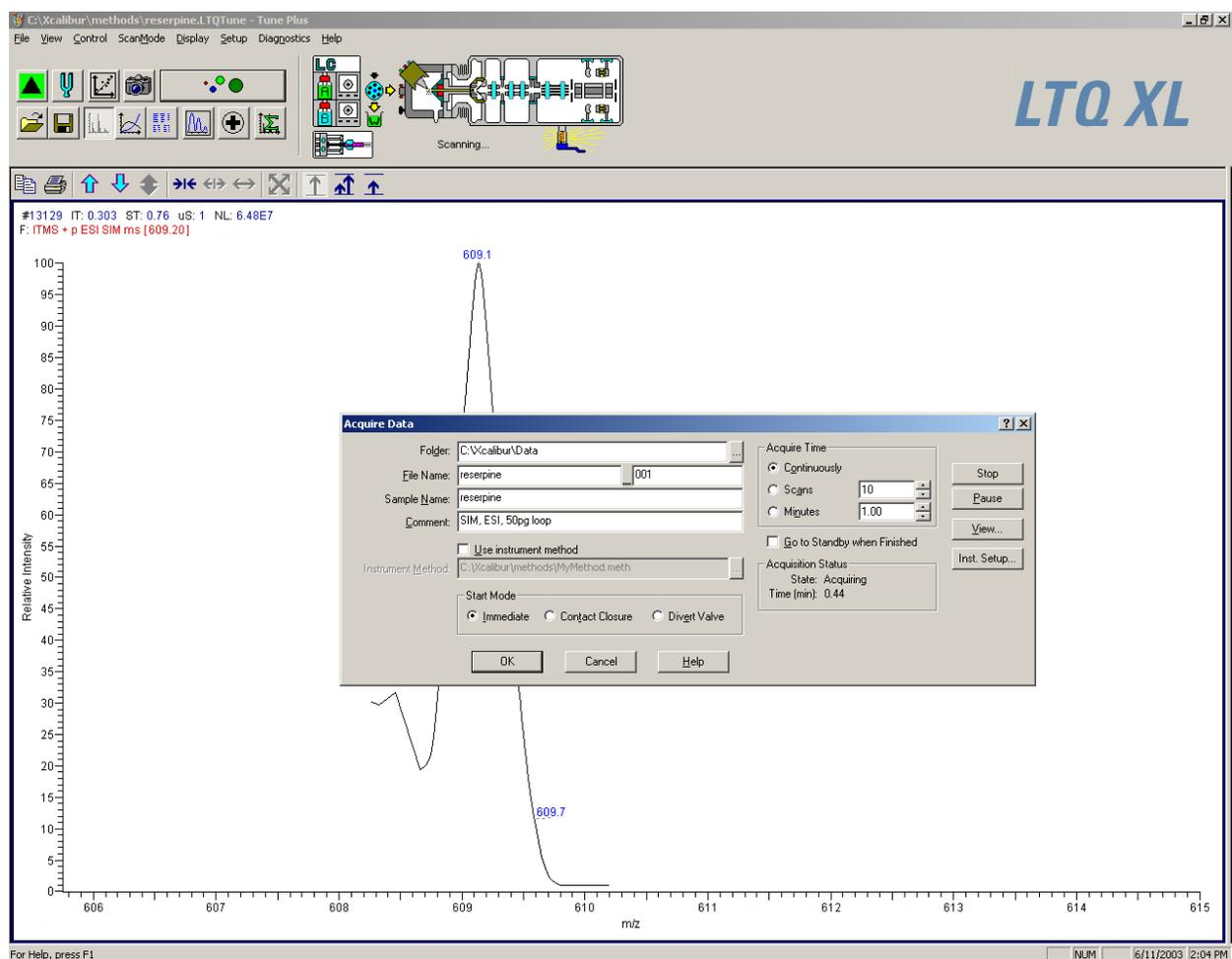
**Figure 48.** Tune Plus window, showing the SIM spectrum of reserpine during analysis by loop injection
