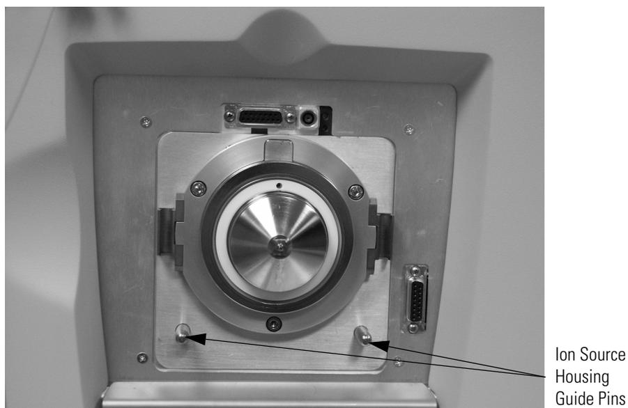
**Figure 54.** Ion source mount showing ion source housing guide pins
