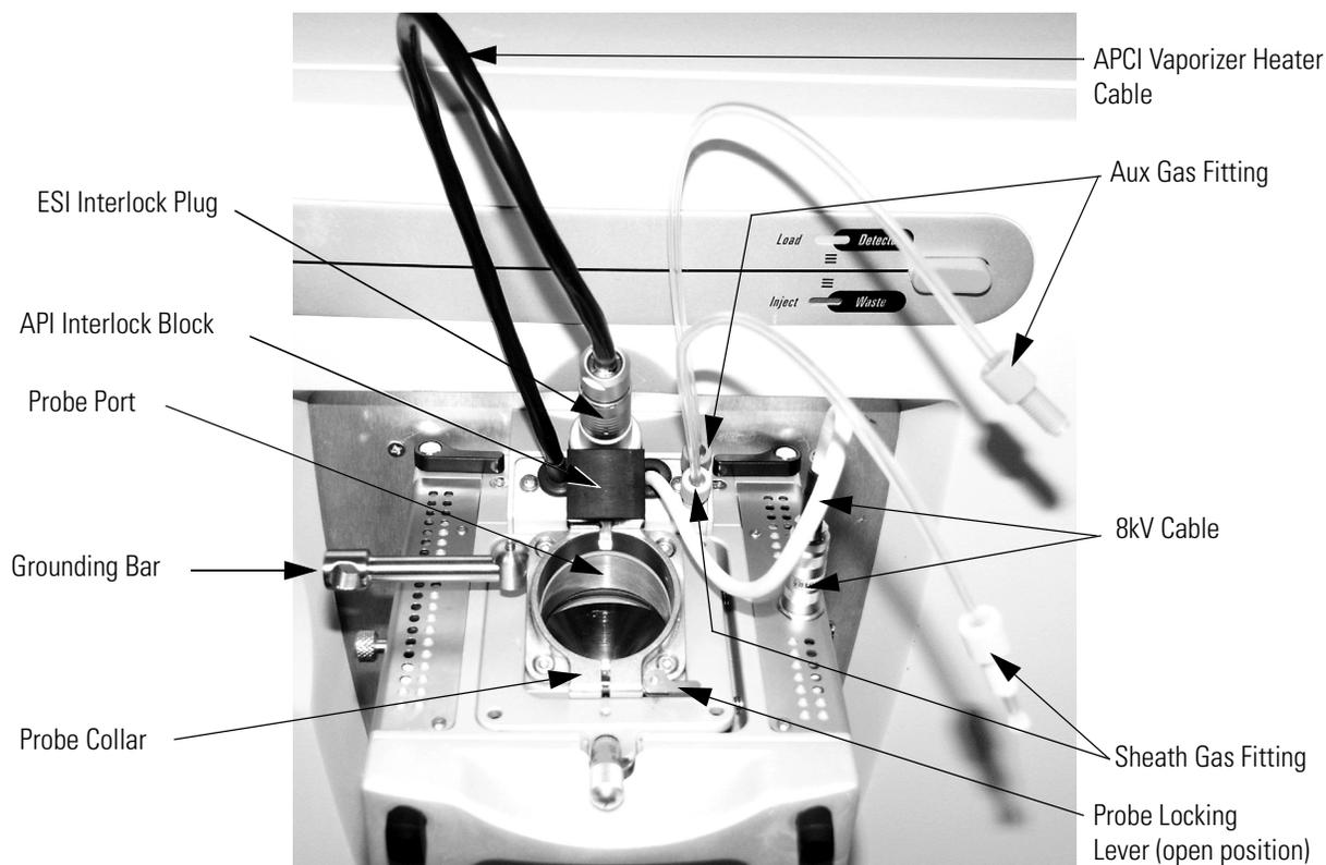
**Figure 13.** Ion Max ion source housing probe locking lever open
