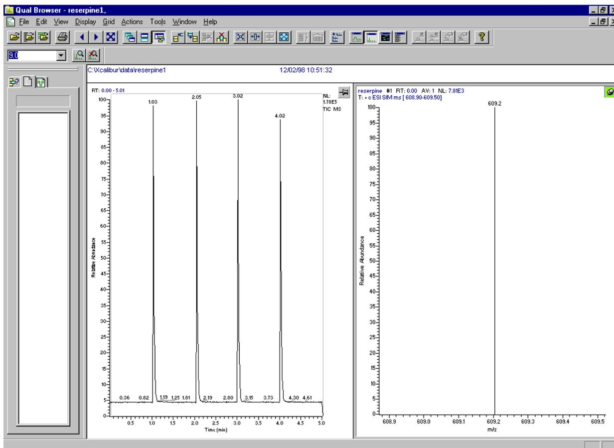
**Figure 49.** Qual Browser window, showing loop injections of reserpine in the Chromatogram view (left) and showing  $m/z$  609 in the Spectrum view. Note that the injections occur at intervals of approximately 1 min
