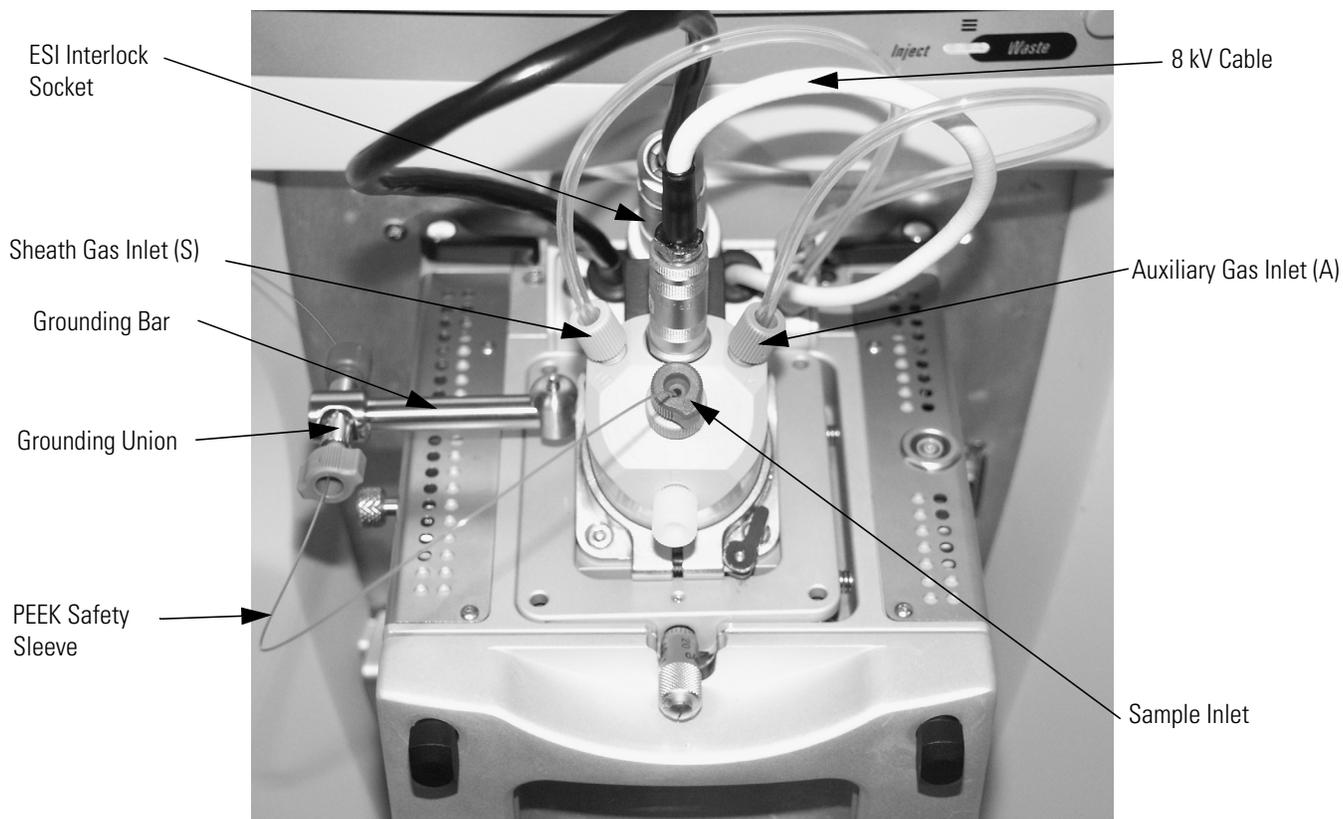
**Figure 15.** Ion Max ion source housing with ESI probe installed
