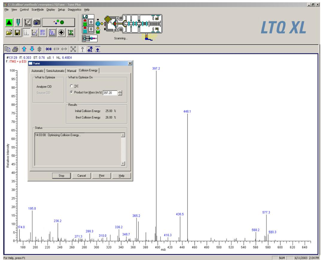
**Figure 41.** Tune Plus window, showing MS/MS product ions of reserpine in the Spectrum view
