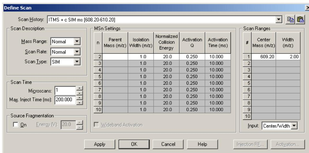
**Figure 65.** Define Scan dialog box, showing typical settings for acquiring data in the SIM scan mode
