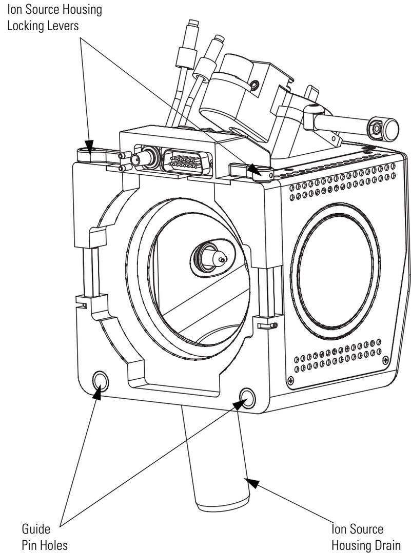
**Figure 53.** Rear view of the Ion Max ion source housing
