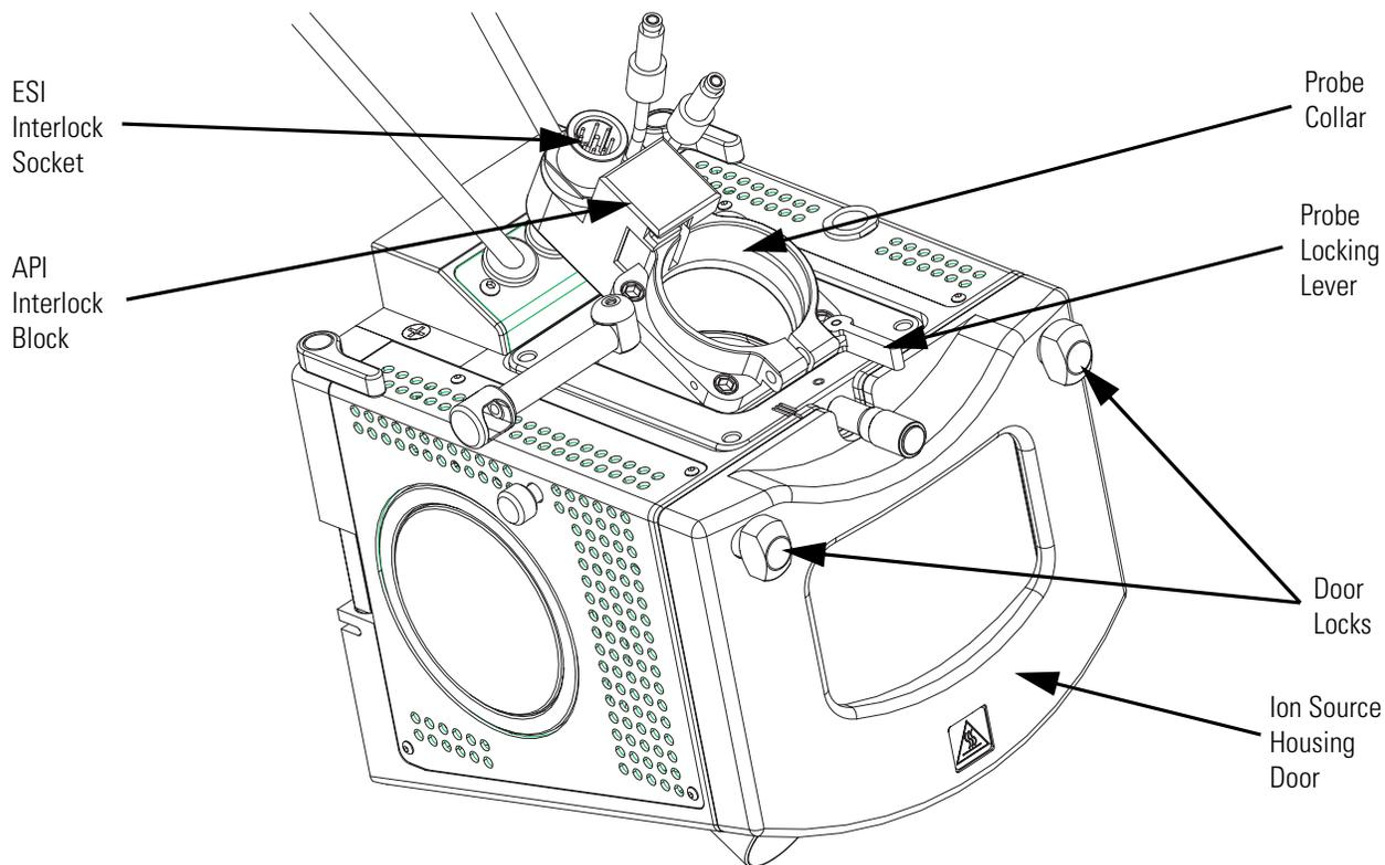
**Figure 6.** Ion Max ion source housing, detail of components
