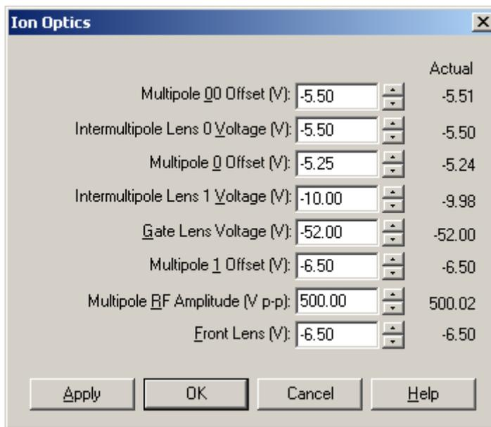
**Figure 26.** Ion Optics dialog box, showing examples of voltages of lenses and Intermultipoles, which are optimized by the LTQ XL automatic tuning procedure
