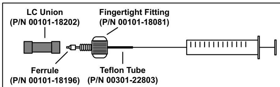
**Figure 56.** APCI/MS plumbing connections for the syringe pump
