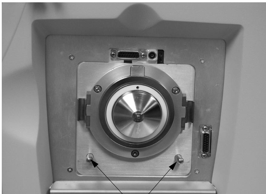
Ion Source Housing Guide Pins
