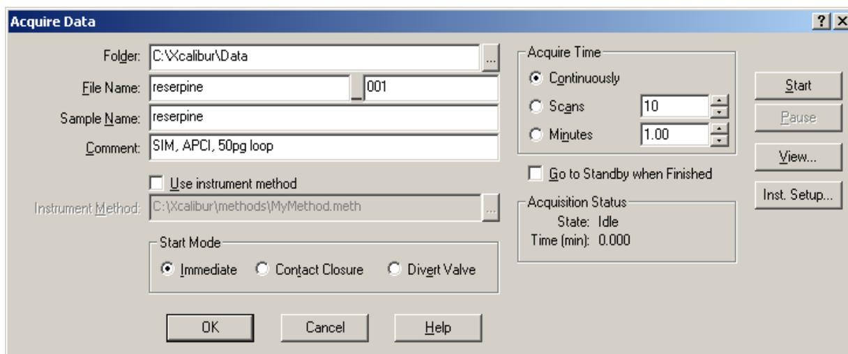
**Figure 46.** Acquire Data dialog box, showing typical settings for acquiring data
