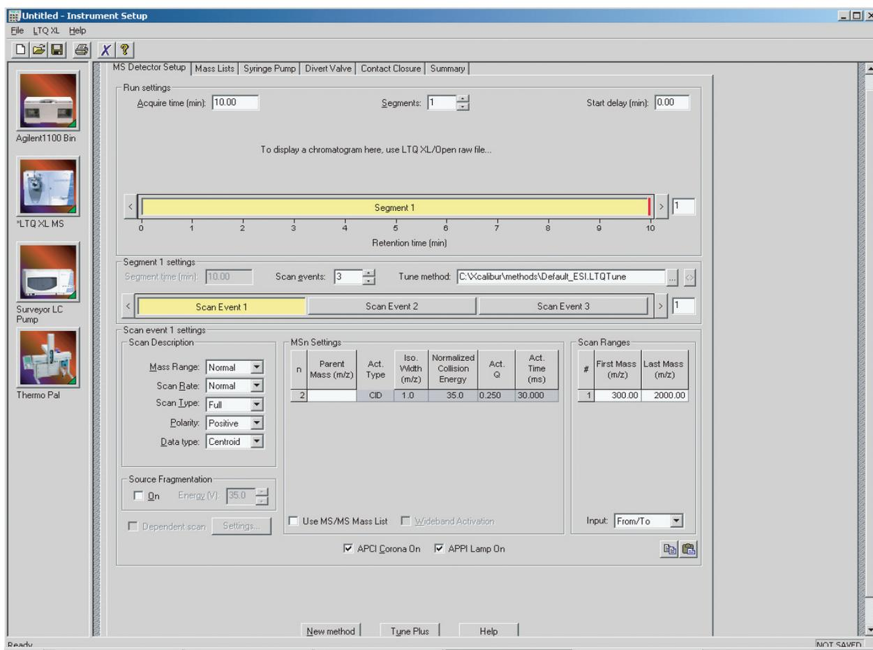
**Figure 2.** MS Detector Setup page in Instrument Setup, showing a template for a Data-Dependent Triple Play experiment. (To select a scan event that makes active the Dependent Scan check box, click either the Scan Event 2 or Scan Event 3 button.)
