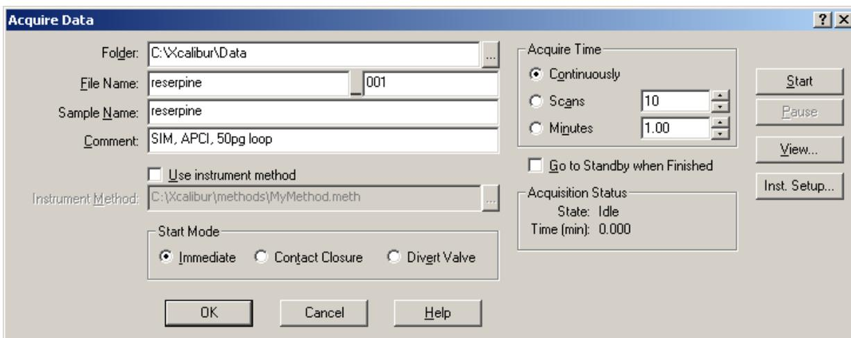
**Figure 66.** Acquire Data dialog box, showing the acquisition status of the raw data file
