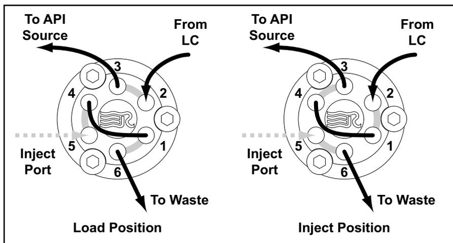
**Figure 63.** Divert/Inject valve, showing the correct setup for analysis by loop injection and showing the flow of liquid through the valve in the Load and Inject positions
