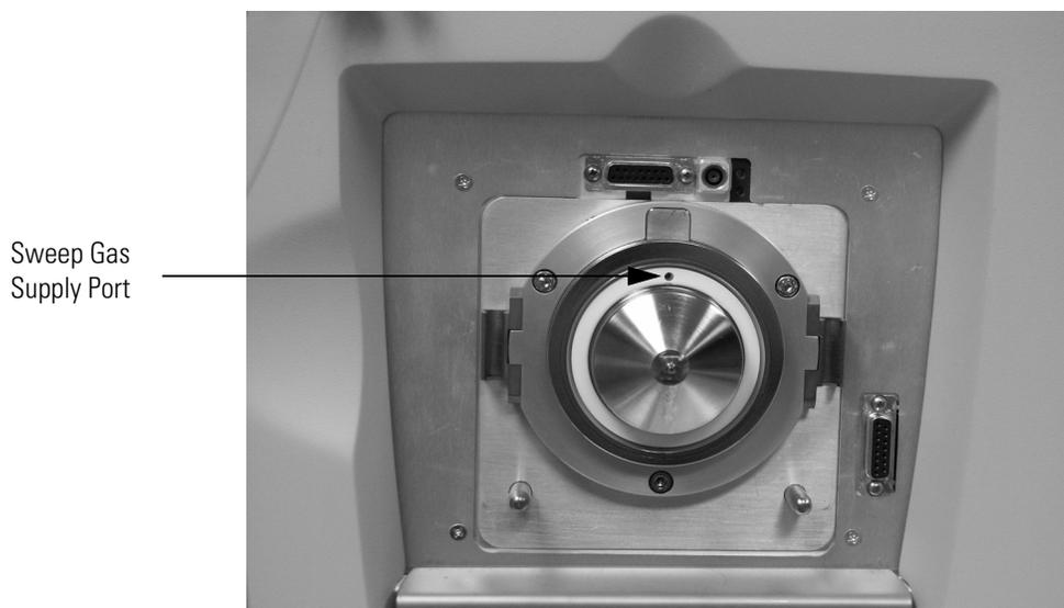
**Figure 9.** Sweep gas supply port in the API cone seal
