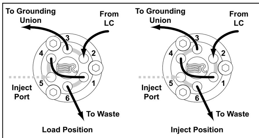
**Figure 44.** Divert/Inject valve, showing the correct setup for analysis by loop injection and showing the flow of liquid through the valve in the Load and Inject positions
