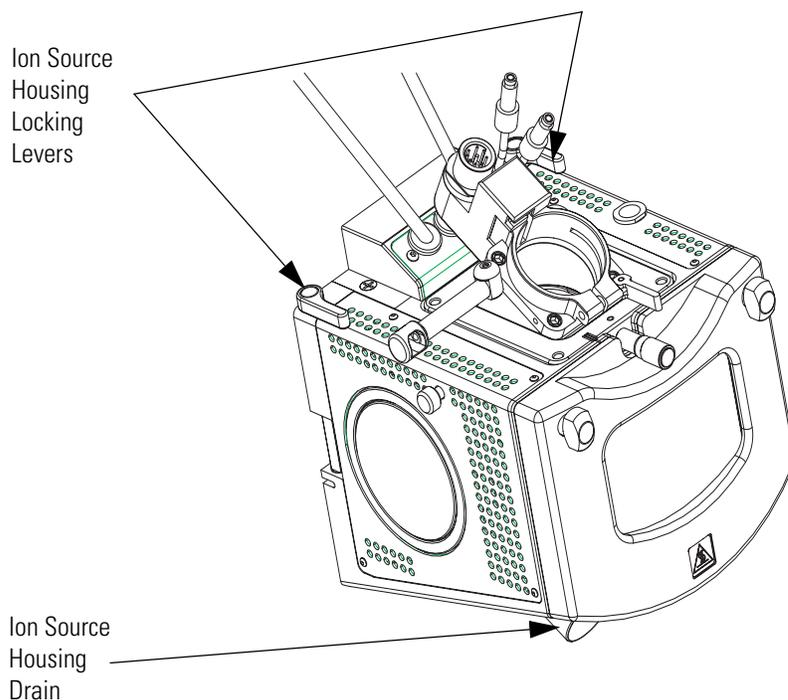
**Figure 8.** Ion Max ion source housing, detail of components
