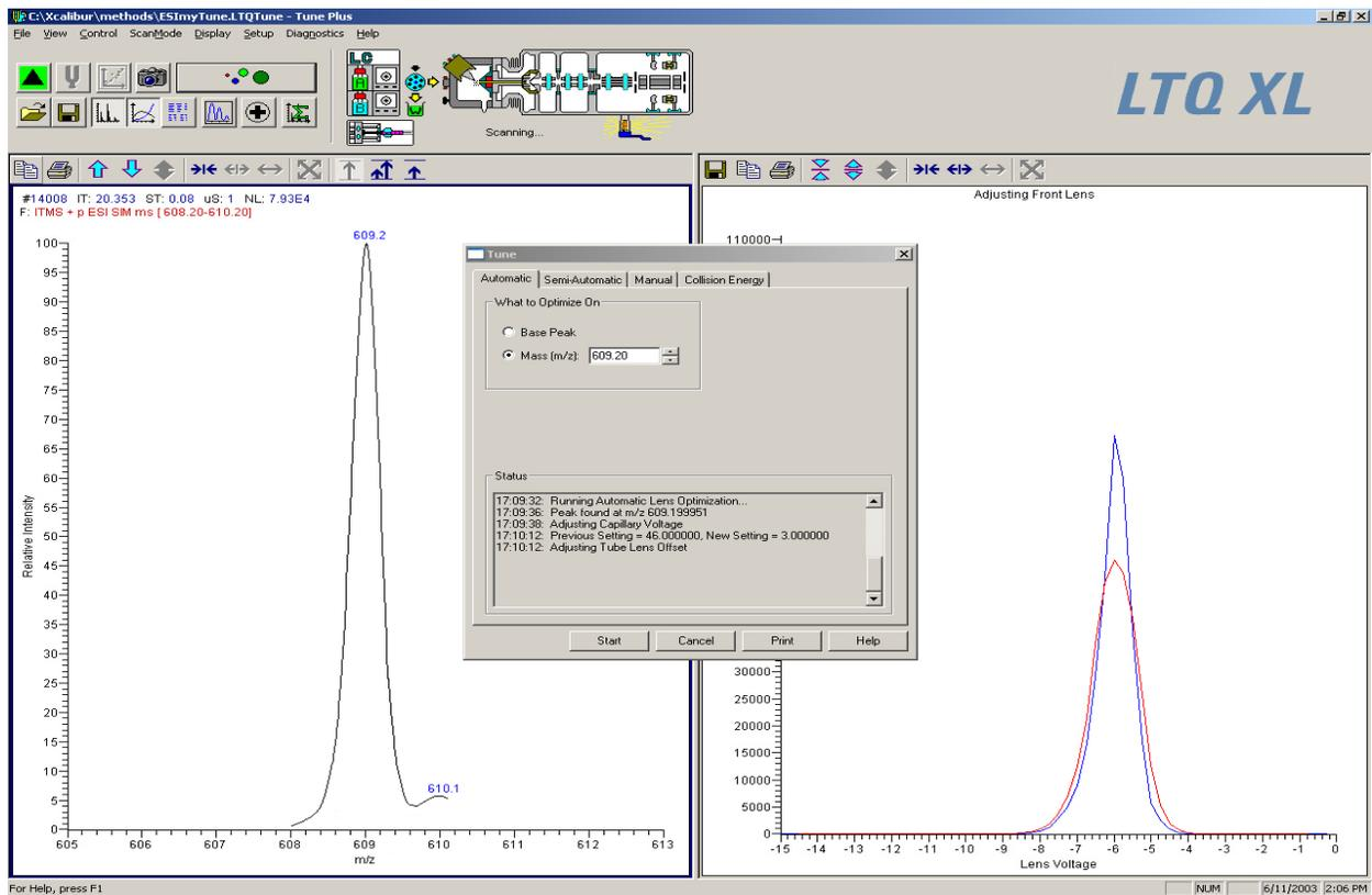
**Figure 35.** Tune Plus window with the Tune dialog box, showing the Automatic tuning page
