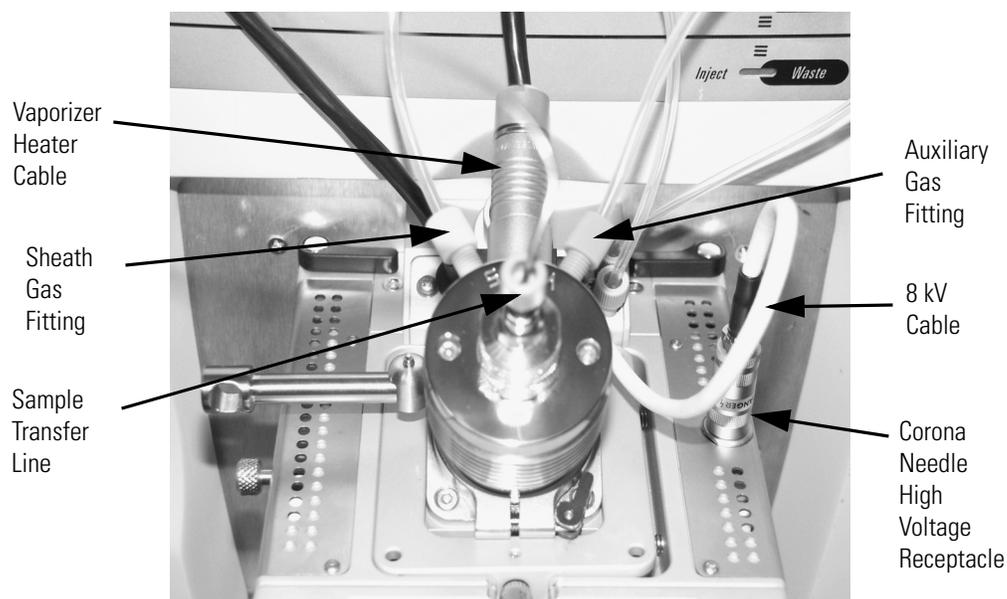
**Figure 5.** Ion Max ion source housing with APCI probe installed
