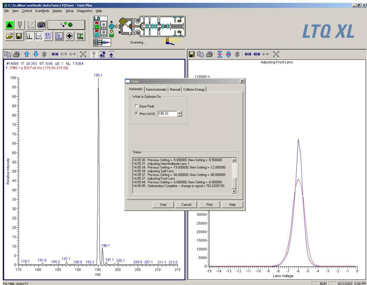
Figure 24. Tune Plus window, showing the results of a typical automatic tune procedure
