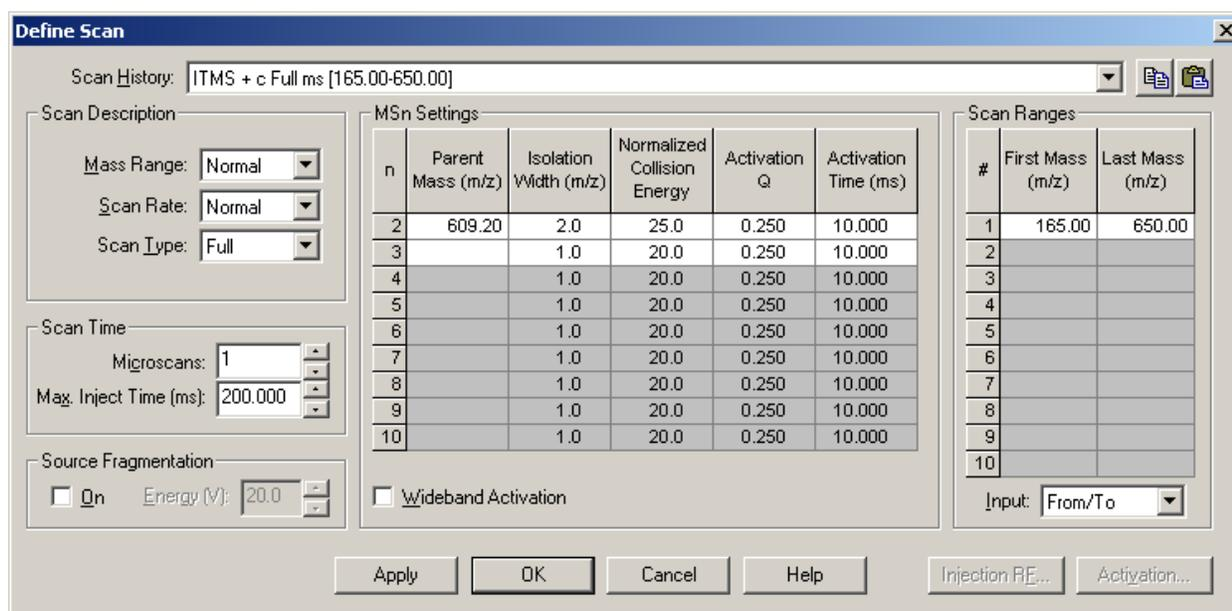
**Figure 39.** Define Scan dialog box, showing typical settings for acquiring MS/MS data in the Full scan type on reserpine
