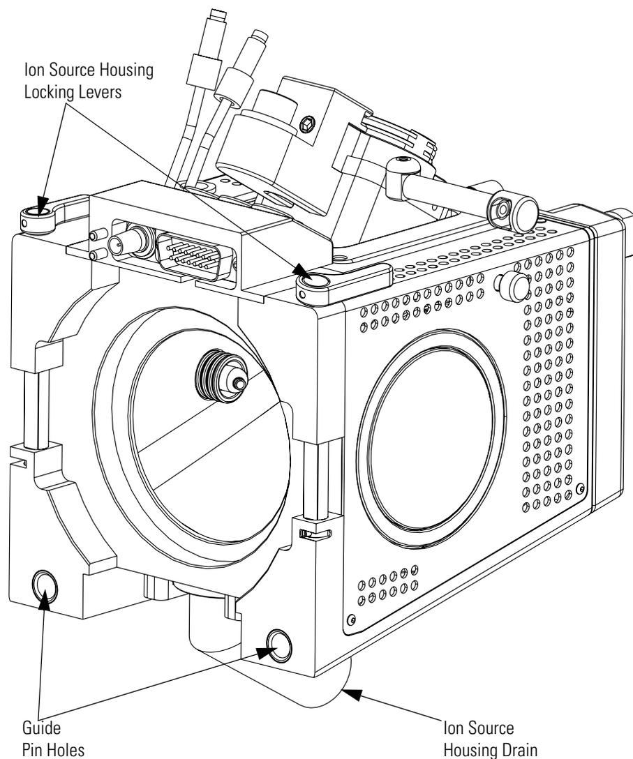
**Figure 11.** Rear view of the Ion Max ion source housing
