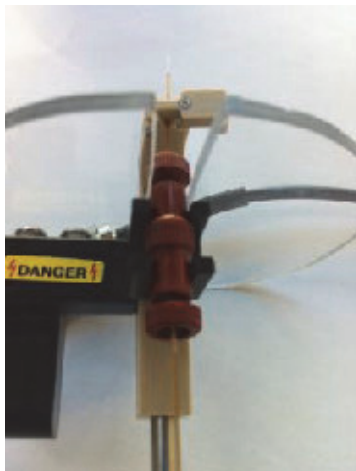
Figure 74. PEEK connector used to secure a long analytical column
