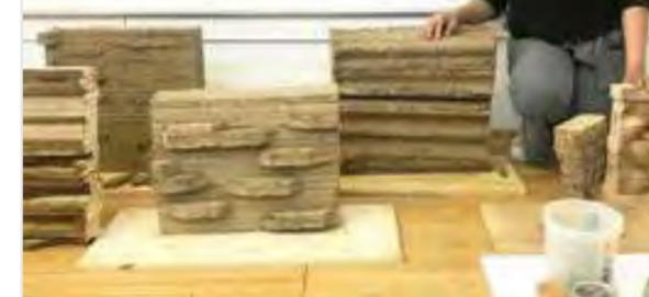
*Thermal mass concrete prototypes optimizing convection through surface figuration, produced in collaboration with industry partner Takl as part of Robotic profiling for concrete surface forming in collaboration with professor Joshua Bard.*
