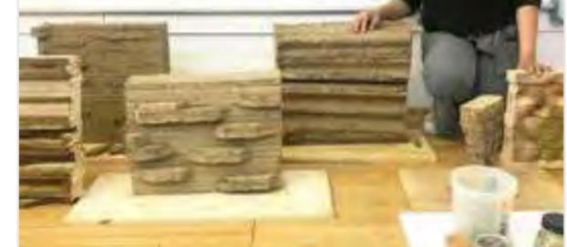
*Thermal mass concrete prototypes optimizing convection through surface figuration, produced in collaboration with industry partner Takl as part of Robotic profiling for concrete surface forming in collaboration with professor Joshua Bard.*
