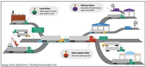
Figure 7.3 Schematic of the transfer hub model for autonomous long-haul trucking. From Viscelli (2020).<sup>248</sup>
