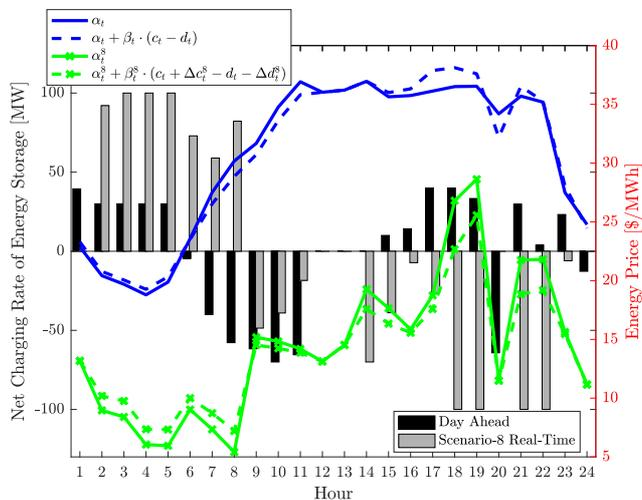
Fig. 5: Day-Ahead and Real-Time Scenario-8 Dispatch of Energy Storage in the Case Study in Section 4 With  $\gamma = 0.70$
