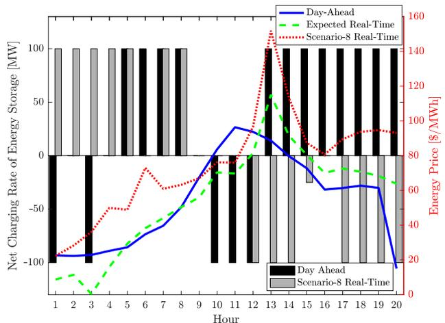
Fig. 2: Day-Ahead and Real-Time Scenario-8 Dispatch of Energy Storage in Base Case of the Example in Section 3 With  $\beta_t = \beta_t^\omega = 0, \forall t \in T, \omega \in \Omega$  and  $\gamma = 1$
