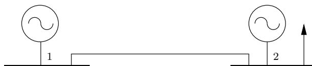
Figure 1: Two-Node, Single-Line Transmission Network for Transmission-Representation Example
