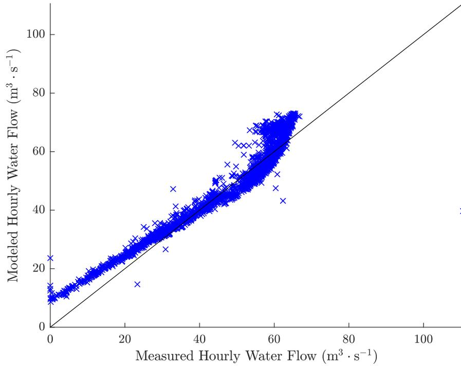
**Fig. 3** Scatter plot of modeled water flow using (5) and actual water flow using 20% of historical data
