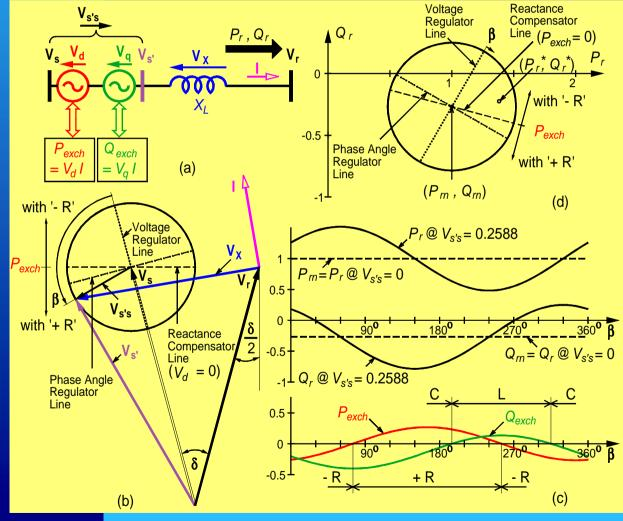
Active and reactive power flow in the line is regulated independently.
