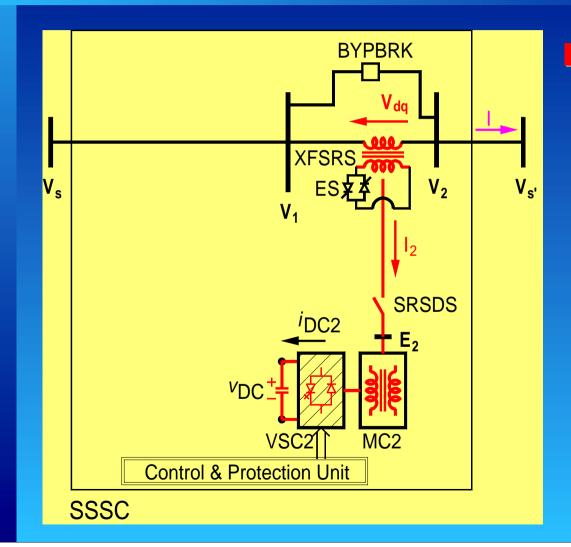
Regulates the transmission line's effective reactance by connecting a compensatng voltage in series with the line and in quadrature with the prevailing line curretnt.
