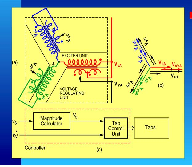
Regulates the line voltage in small steps by adding or subtracting a compensatng voltage in series with the transmission line.
