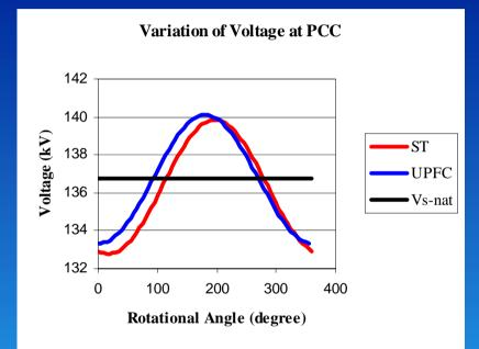
From 205° to 335°, an ST maintains a higher line voltage than a UPFC.
