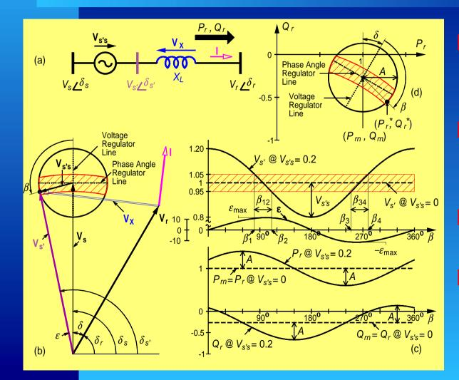
Line voltage is bounded by ±5% over nominal voltage. Full range of voltage injection is not permitted. Full capability of a UPFC is not utilized. ST can be modified to fit customers' needs.
