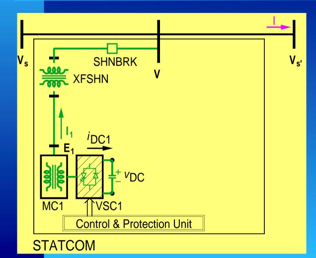
Regulates the line voltage by injecting a shunt reactive current into the transmission line.
