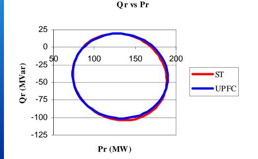
Area of controllability in the P-Q plane for an ST and a UPFC are almost identical.
