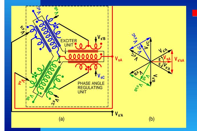
Regulates the phase angle of the line voltage by a seriesconnected compensating voltage that is in quadrature with respect to the line voltage.
