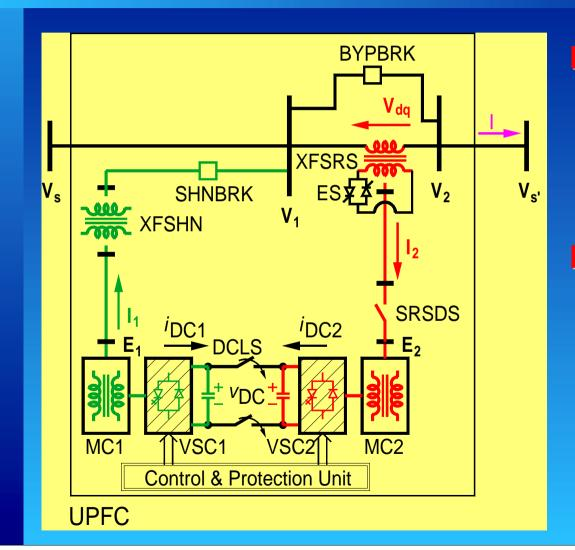
Regulates the active and the reactive power flow in the line independently. Regulates the line voltage by injecting a shunt reactive current into the transmission line.
