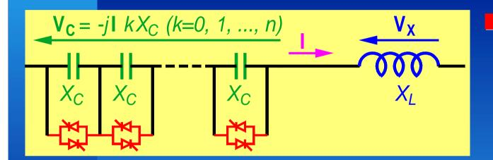
Regulates the transmission line's effective reactance by connecting a capacitor, parallel with a bypass switch, in series with the transmission line.
