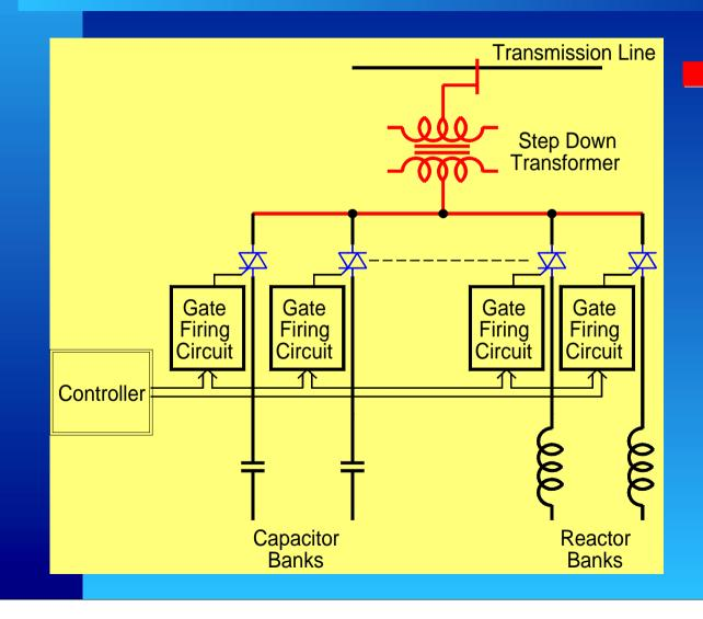
Regulates the line voltage by connecting an inductor or a capacitor in parallel with the transmission line.
