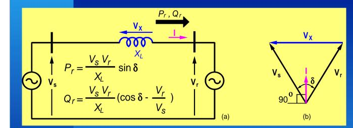
Power flow in a transmission line depends on
