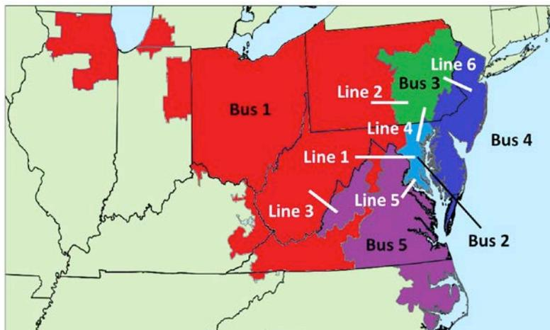
**Fig. 1** Reduced form model of the PJM Interconnection
