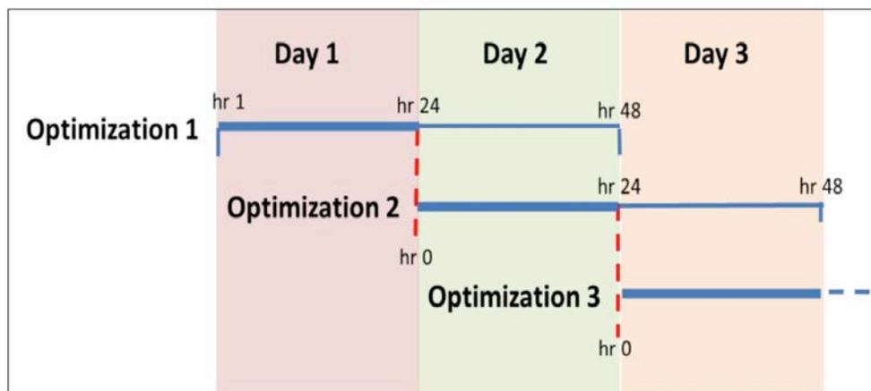
**Fig. 12** Illustration of how PHORUM handles day boundaries. Each optimization runs for a full 48 hours, but only the first 24 hours of results are retained. Variables are passed from the 24<sup>th</sup> hour of the first optimization to hour 0 of the second.
