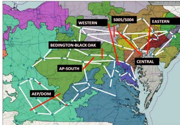
**Fig. 10** PJM 500kV transmission lines (white lines) and transmission interfaces (red lines) [40, 41]. Most interfaces contain multiple 500kV lines
