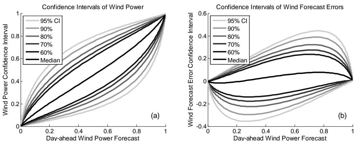
Figure 7: ERCOT wind power confidence levels (left plot) based on wind forecast level and wind error confidence levels (right plot) based on wind forecast level.
