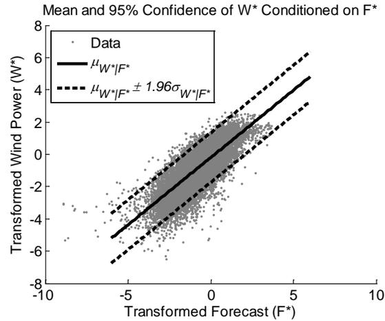
Figure 5: Transformed ERCOT data with conditional mean for  $W^*$  and 95% confidence interval of  $W^*$  as a function of  $F^*$ .
