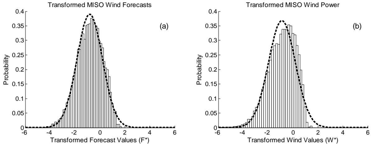
Figure 10: Relative frequency distributions (histogram bars) for the transformed wind power forecast (a) and wind power (b) in ERCOT with a fitted normal distribution (dashed line) overlaid.
