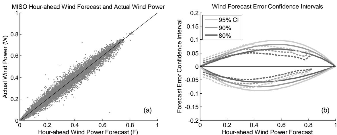
Figure 13: MISO wind power plotted against the hour-ahead persistence forecasts (a), and confidence intervals for wind forecast errors (b). Solid lines are calculated using the logit transformation, and dashed lines are calculated with a moving window.
