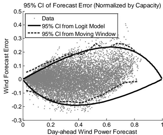
Figure 11: Wind forecast errors in MISO plotted against wind forecast values with 95% confidence intervals. Solid lines are calculated using the logit transformation, and dashed lines are calculated with a moving window of width 0.1.
