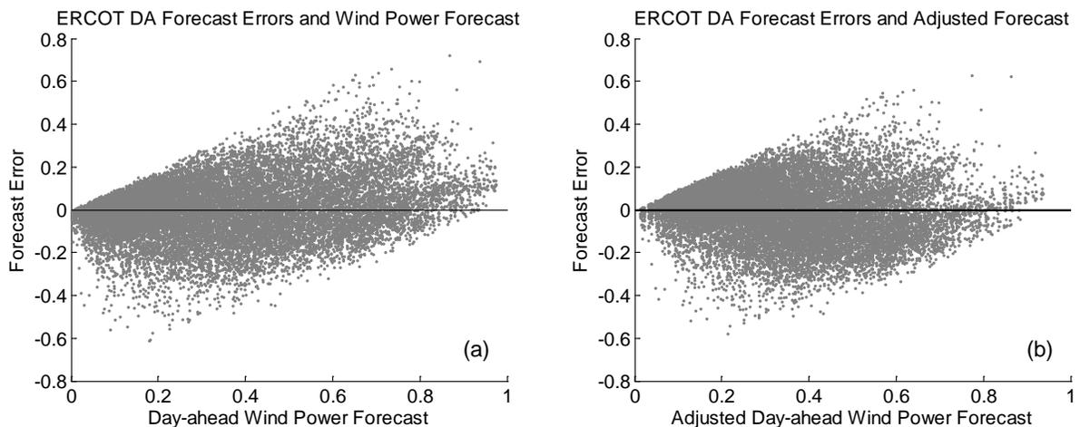
Figure C.3: Wind forecast error distributions from ERCOT with original data (a) and with the conditional bias removed from the forecasts.
