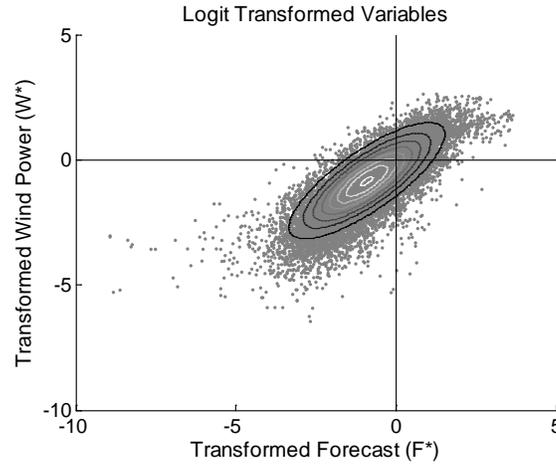
Figure 4: Logit transformed wind power data plotted against transformed wind forecast data. The data shown here are transformations of the data displayed in Figure 1 (a). Solid lines are contours of a fitted bivariate normal distribution with  $\mu_{F^*} = -0.74$ ,  $\mu_{W^*} = -0.81$ ,  $\sigma_{F^*} = 1.55$ ,  $\sigma_{W^*} = 1.70$  and  $\rho = 0.80$
