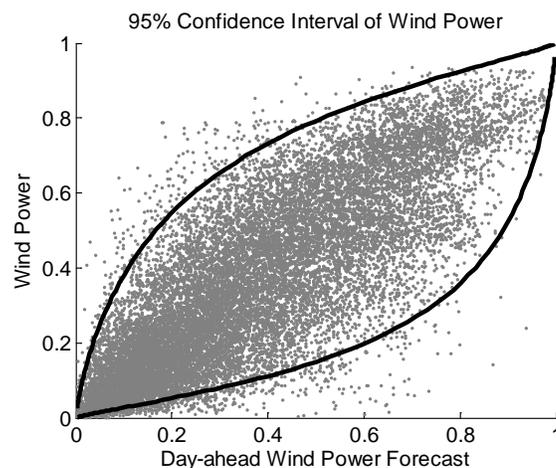
Figure 6: Ninety-five percent confidence interval for estimated uncurtailed ERCOT wind power in the original space plotted as a function of the day-ahead forecast level of wind power.
