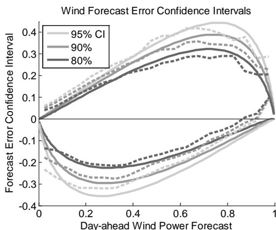
Figure 8: Confidence intervals conditioned on ERCOT wind forecast level. Solid lines are calculated using the logit transformation, and dashed lines are calculated by binning data according to the forecasts.
