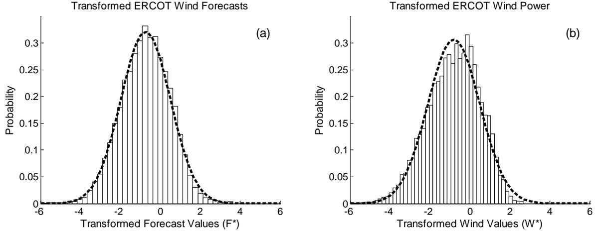
Figure 3: Relative frequency distributions (histogram bars) for the transformed wind power forecast (a) and wind power (b) in ERCOT with a fitted normal distribution (dashed line) overlaid. Analogous MISO data are shown in Figure 10.
