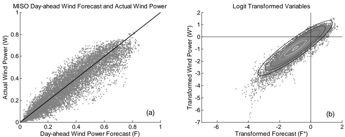
Figure 9: (a) Actual wind power in MISO plotted against the day-ahead forecast values and (b) the logit transformation of the same data. A contour (solid lines) of the fitted bivariate normal distribution is plotted over the data in (b) with  $\mu_{F^*} = -0.82$ ,  $\mu_{W^*} = -0.89$ ,  $\sigma_{F^*} = 1.05$ ,  $\sigma_{W^*} = 1.18$  and  $\rho = 0.92$
