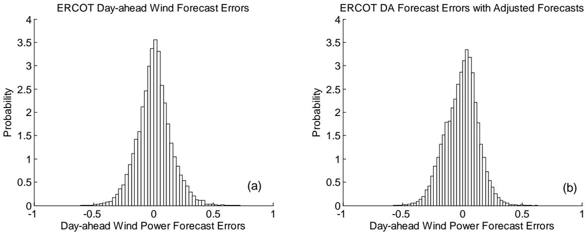
Figure C.2: Wind forecast error distributions from ERCOT with original data (a) and with the conditional bias removed from the forecasts.
