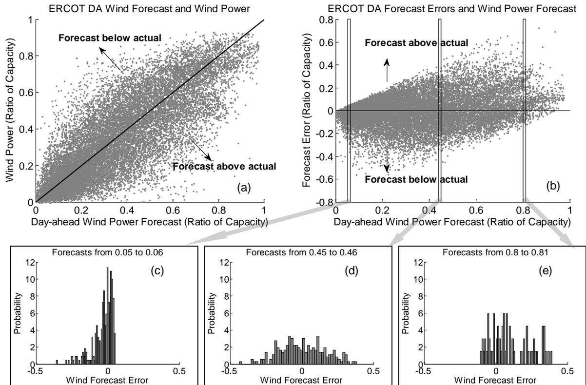
Figure 1: ERCOT Estimated uncurtailed wind power (a) and wind forecast errors (b) plotted against forecast wind power. Bottom plots show probability distributions of wind forecast errors corresponding to the three bins highlighted in the (b). Forecast value ranges in the bottom plots are (c) 0.05 to 0.06, (d) 0.45 to 0.46 and (e) 0.8 to 0.81. All values are shown as ratios of installed wind capacity.
