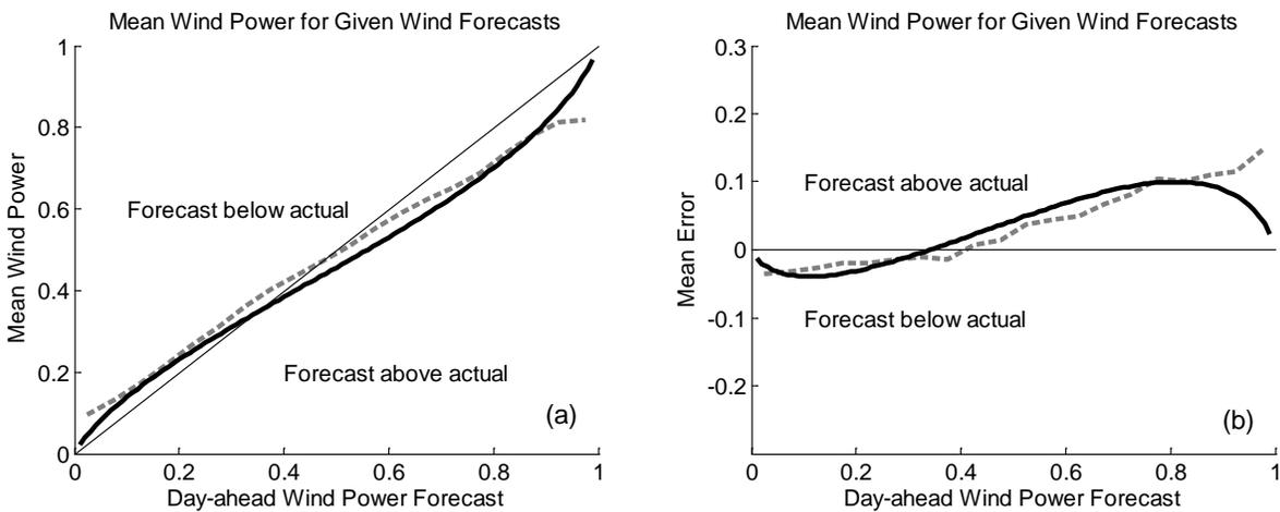
Figure C.1: Mean wind power conditioned on the wind power forecast (a) and mean forecast error conditioned on the wind power forecast (b). Solid lines were calculated directly with binned data, and dashed lines were calculated using the logit-normal distribution.
