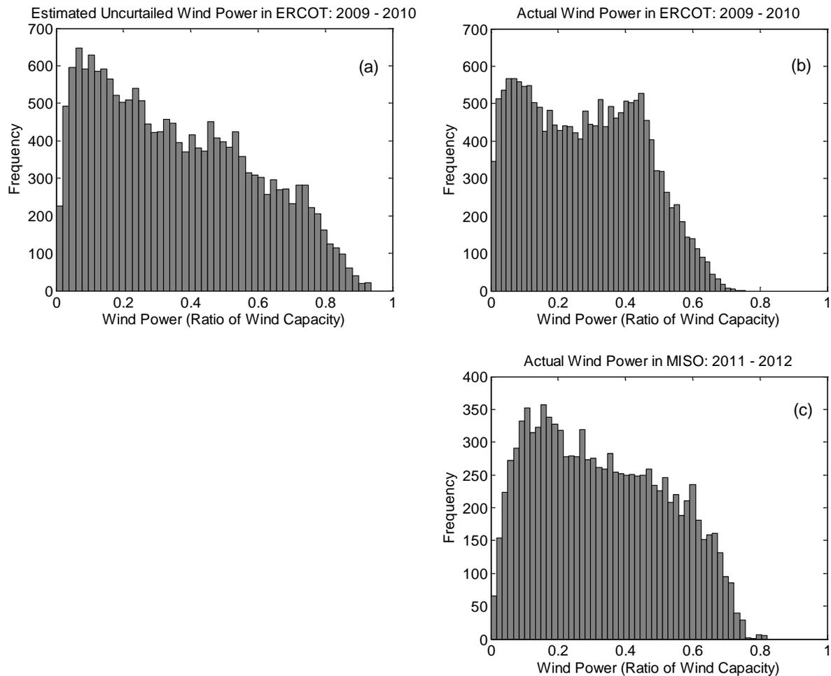
Figure A.1: Frequency distributions of (a) uncurtailed hourly wind power in ERCOT (b) actual hourly wind power in ERCOT and (c) actual hourly wind power in MISO.
