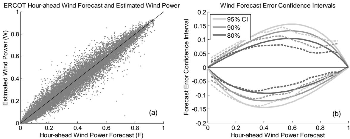
Figure 12: ERCOT estimated uncurtailed wind power plotted against the hour-ahead persistence forecasts (a), and confidence intervals for wind forecast errors (b). Solid lines are calculated using the logit transformation, and dashed lines are calculated with a moving window.
