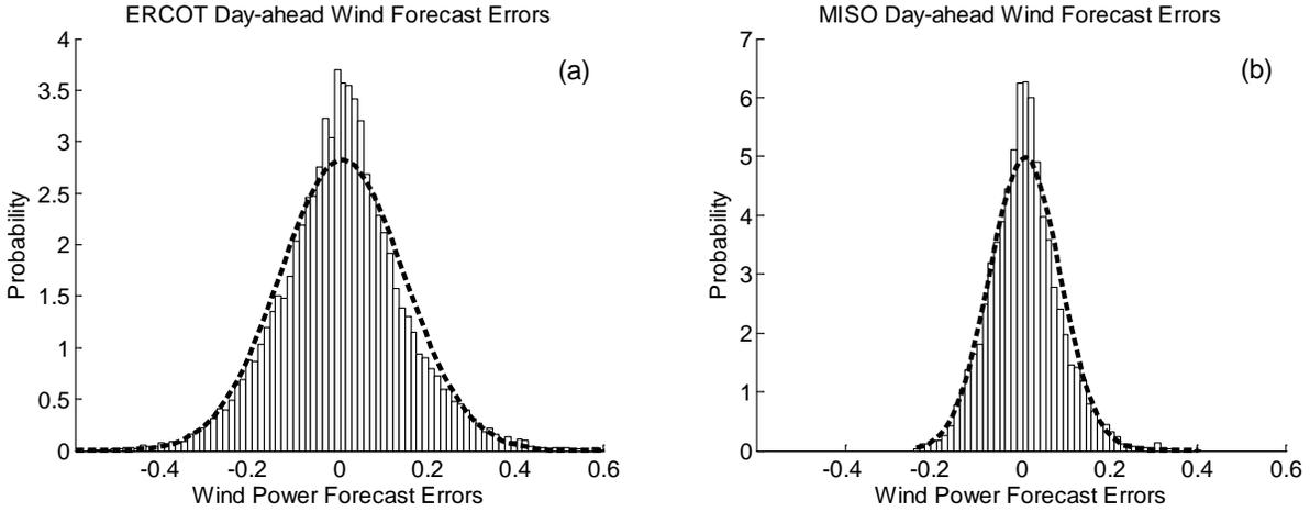
Figure A.2: Frequency distribution (histogram bars) of wind power forecast errors in ERCOT (a) and MISO (b) with a fitted normal distribution (dashed line) overlaid.
