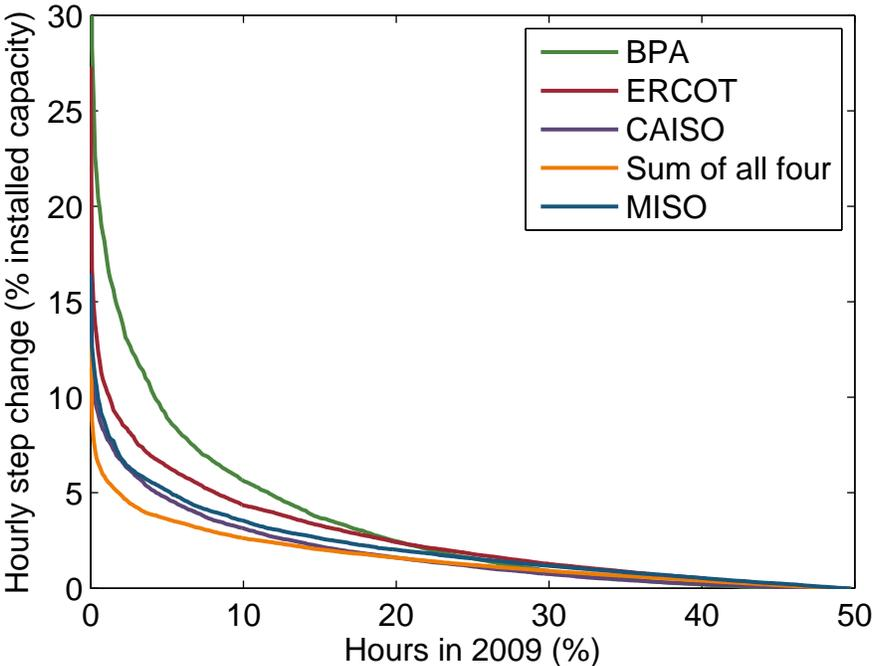
Figure S2: Duration curve for hourly step changes. BPA and ERCOT are the most likely to have large hourly step changes, and MISO and the interconnected regions are the least likely. For clarity, the curve shows only positive step changes; the negative portion of the curve is roughly symmetrical.
