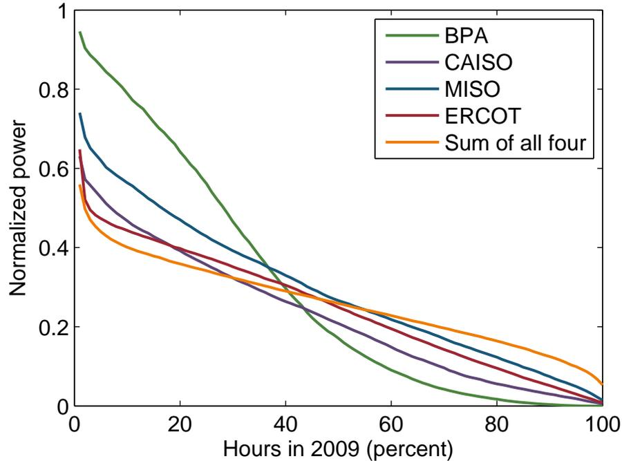
Figure 4: Duration curve for 2009 wind power output. The interconnected regions show the greatest percentage of firm power (capacity available 79 to 92 % of the time) and BPA the least.
