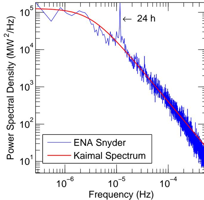
Figure S1: Kaimal approximation to the PSD of 15-minute wind energy data from a single 63 MW wind plant in Snyder, Texas (ERCOT). The peak at the frequency corresponding to 24 hours is highlighted, showing the strong daily periodicity in the wind power output. The fitted parameters are  $A = 1.27 \times 10^5$  and  $B = 1.47 \times 10^9$ . The PSD was calculated with 16 segment averaging to reduce noise.
