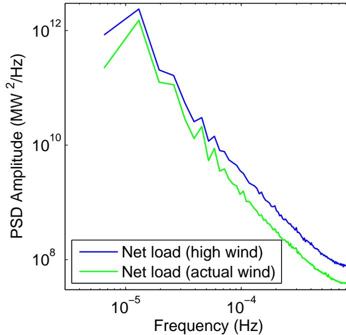
Figure S4: PSDs of 2010 CAISO net load with historical wind power output and wind power output amplified by a factor of 10. Increased wind capacity raises net load variability evenly across frequencies. PSDs are calculated with 16 averaging segments.
