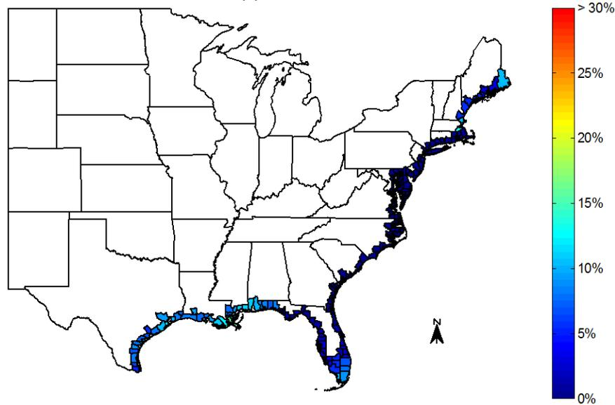
Figure 2: Probability that hurricanes destroy more than 10% of a wind farm in 20 years if the turbines have backup power for the yaw motors so they can track the wind direction. Results for individual counties are listed in Table 3 in the column labeled “yawing”.
