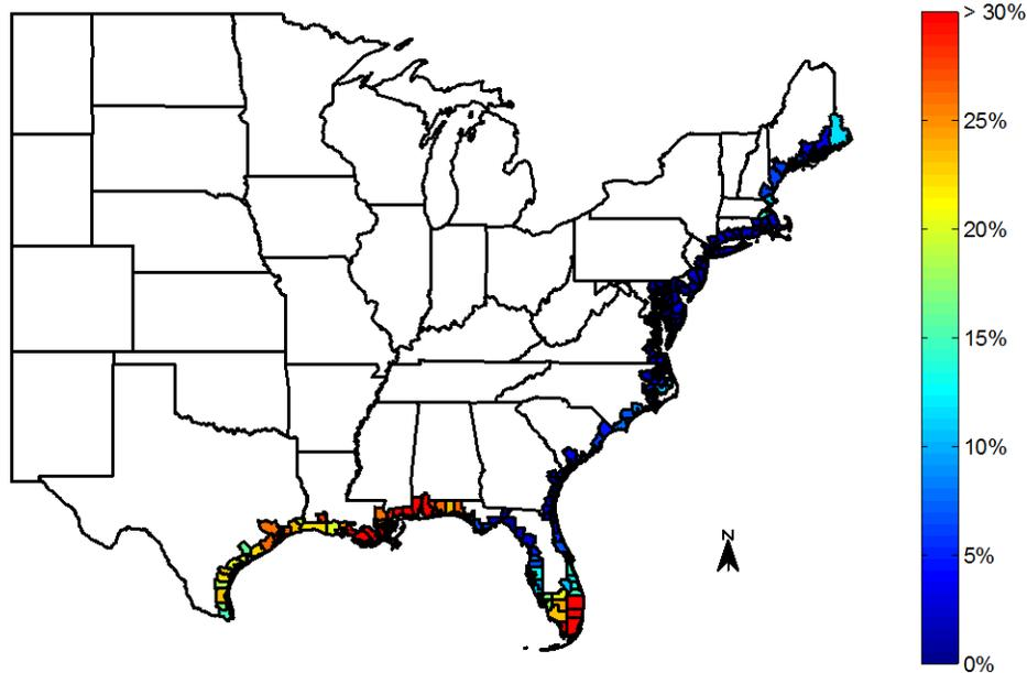
Figure 1: Probability that hurricanes destroy more than 10% of a wind farm in 20 years if the turbines cannot yaw to track the wind direction. Results for individual counties are listed in Table 3 in the column labeled “no yaw”.
