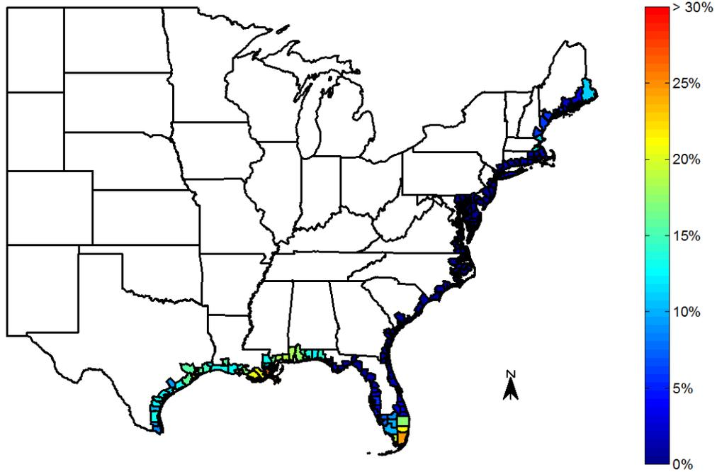
Figure 4: Probability that hurricanes destroy more than 50% of a wind farm in 20 years if the turbines cannot yaw to track the wind direction. These results are similar to the results in Figure 1, but show the probability that of higher damage to the wind farm.
