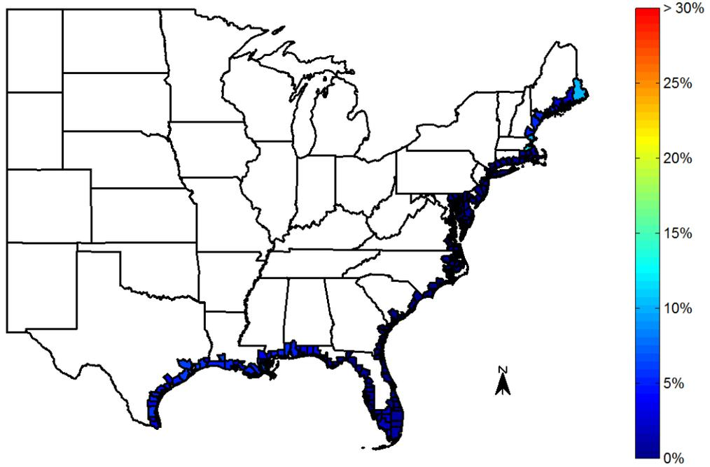
Figure 5: Probability that hurricanes destroy more than 50% of a wind farm in 20 years if the turbines have backup power for the yaw motors so they can track the wind direction. These results are similar to the results in Figure 2, but show the probability that of higher damage to the wind farm.
