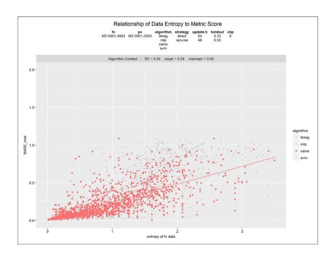
**Figure 3-8:** Best metric score vs. entropy, naive. Data sources from the M3 Forecasting Competition. 3,003 data sources from x 32 techniques = 96,096 forecasts and evaluations. Evaluation by MASE score. Entropy values are arranged along the x-axis. *Red* is best technique applied to one data source, filtered for naive algorithm class.
