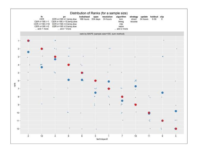
**Figure 5-13:** Effect of sampling – distribution of technique ranks across samples vs. technique at sample size 195, Ireland, week-ahead forecasts. 12 techniques. Metric is MAPE. *Blue* is technique rank for a specific technique applied to 1 of 10 samples of size 195 out of 782. *Large blue* is mean technique rank for a specific technique applied to all 10 samples. *Large red* is technique rank for a specific technique applied to full population.
