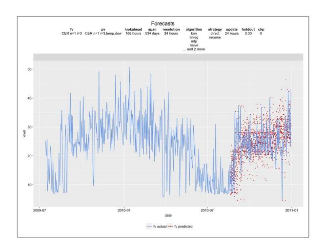
**Figure 5-6:** Effect of sampling – forecasts, Ireland, week-ahead forecasts. 12 techniques. *Blue* is electricity usage/demand series for a specific sample of size 1 out of 782. *Red* is overlay of 12 forecasts of the specific sample.
