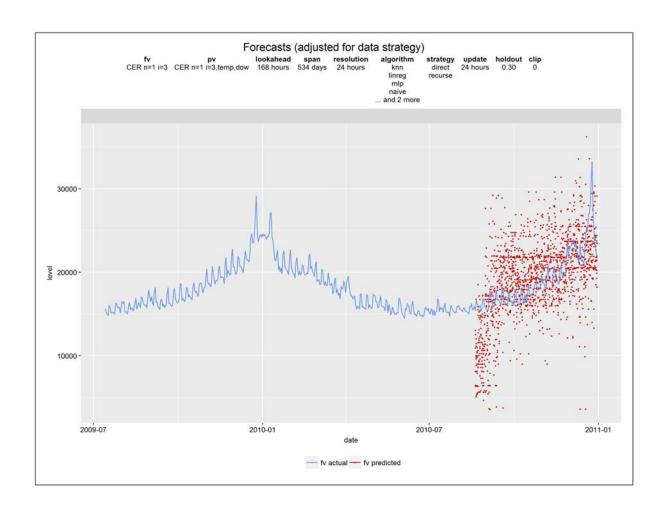
**Figure 5-7:** Effect of sampling – forecasts, Ireland, week-ahead forecast. *Blue* is electricity usage/demand series for the population. *Red* is overlay of 12 forecasts of a specific sample of size 1 out of 782 re-scaled to the population size.
