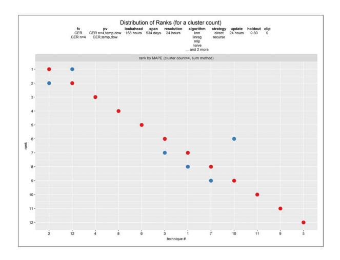
**Figure 5-23:** Effect of clustering – technique rank vs. technique at 4 clusters, Ireland, week-ahead forecasts. 12 techniques. Metric is MAPE. *Blue* is technique rank for a specific technique applied when grouping as 4 clusters. *Red* is technique rank for a specific technique applied without clustering.
