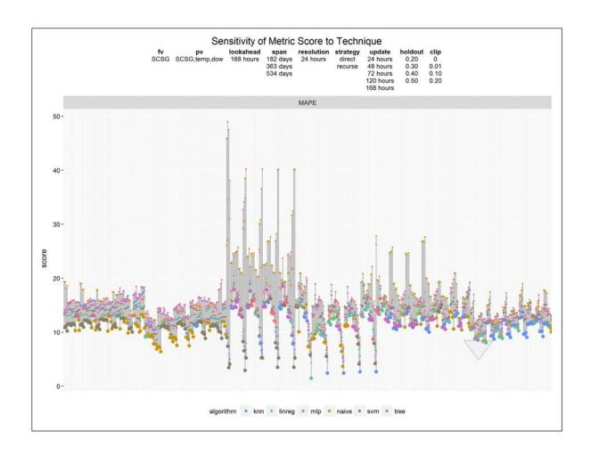
**Figure 6-8:** <u>Distribution of metric scores across techniques, Australia, week-ahead forecasts.</u> 2,880 techniques and forecasts. Each vertical bar represents a family of techniques that differ from each other only by algorithm class. Distances along the vertical bars represent metric scores for specific techniques. Metric is MAPE. *Colors* are algorithm class. *Large point* is metric score of best technique within a family of techniques.
