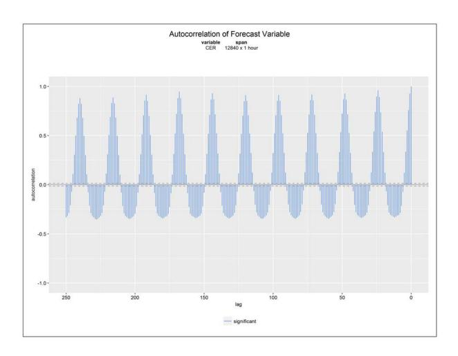
**Figure 4-5:** <u>Autocorrelation of reference series, Ireland, for day-ahead forecasts.</u> Reference series is aggregate electricity usage.
