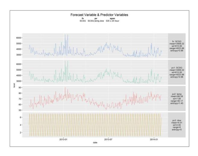
**Figure 6-3:** Reference and predictor series, Australia, for week-ahead forecasts. Reference series is aggregated 223-household electricity usage. Predictor series are aggregate electricity usage, temperature, and day of week (integer coded).
