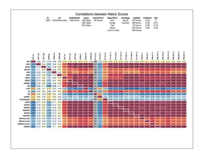
**Figure 4-45:** Correlations of scores per one standard metric-to-scores per one penalty metric, across metric pairs, Ireland, week-ahead forecasts. 2,880 techniques and forecasts. For each cell, all techniques are scored per two metrics, and the sequence of scores per the first metric are correlated with the sequence of scores per the second metric. *Red* is positive correlation. *Blue* is negative correlation. *Dark* is strong absolute correlation. *Light* is weak absolute correlation.
