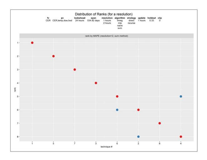
**Figure 5-32:** Effect of temporal magnification — technique rank vs. technique at long time step size, Ireland, day-ahead forecasts. 24 techniques (3 decision options for time step size, 8 combinations of other decision options). Metric is MAPE. *Blue* is technique rank for a specific technique applied at temporal magnification with 2-hour time step size. *Red* is technique rank for a specific technique applied without temporal magnification (baseline 1-hour time step size).
