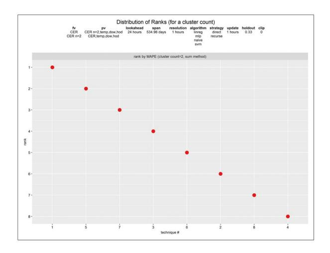
**Figure 5-26:** Effect of clustering – technique rank vs. technique at 2 clusters, Ireland, day-ahead forecasts. 8 techniques. Metric is MAPE. *Blue* is technique rank for a specific technique applied when grouping as 2 clusters (hidden by red). *Red* is technique rank for a specific technique applied without clustering.
