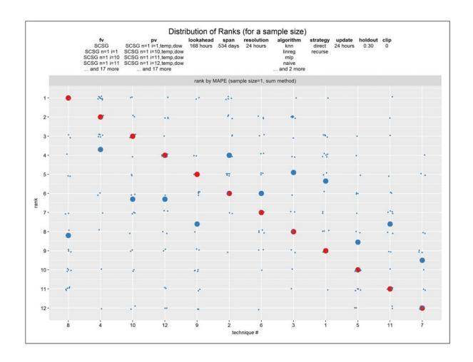
**Figure 6-43:** Effect of sampling – distribution of technique ranks across samples vs. technique at sample size 1, Australia, week-ahead forecasts. 12 techniques. Metric is MAPE. *Blue* is technique rank for a specific technique applied to 1 of 20 samples of size 1 out of 223. *Large blue* is mean technique rank for a specific technique applied to all 20 samples. *Large red* is technique rank for a specific technique applied to full population.
