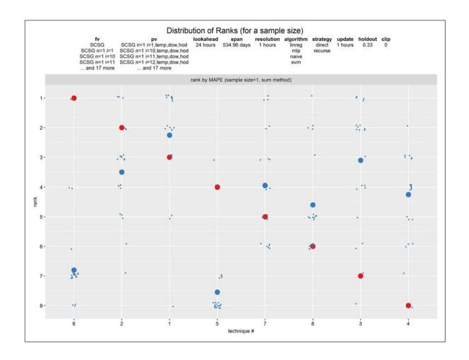
**Figure 6-45:** Effect of sampling – distribution of technique ranks across samples vs. technique at sample size 1, Australia, day-ahead forecasts. 8 techniques. Metric is MAPE. *Blue* is technique rank for a specific technique applied to 1 of 20 samples of size 1 out of 223. *Large blue* is mean technique rank for a specific technique applied to all 20 samples. *Large red* is technique rank for a specific technique applied to full population.
