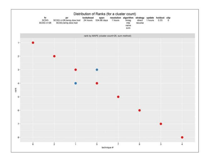
**Figure 6-50:** Effect of clustering – technique rank vs. technique at 26 clusters, Ireland, day-ahead forecasts. 8 techniques. Metric is MAPE. *Blue* is technique rank for a specific technique applied when grouping as 26 clusters. *Red* is technique rank for a specific technique applied without clustering.
