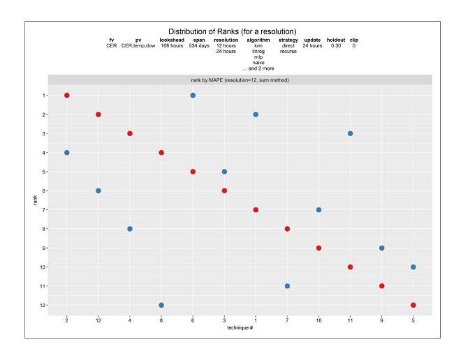
**Figure 5-30:** Effect of temporal magnification — technique rank vs. technique at medium time step size, Ireland, week-ahead forecasts. 36 techniques (3 decision options for time step size, 12 combinations of other decision options). Metric is MAPE. *Blue* is technique rank for a specific technique applied at temporal magnification with 12-hour time step size. *Red* is technique rank for a specific technique applied without temporal magnification (baseline 24-hour time step size).
