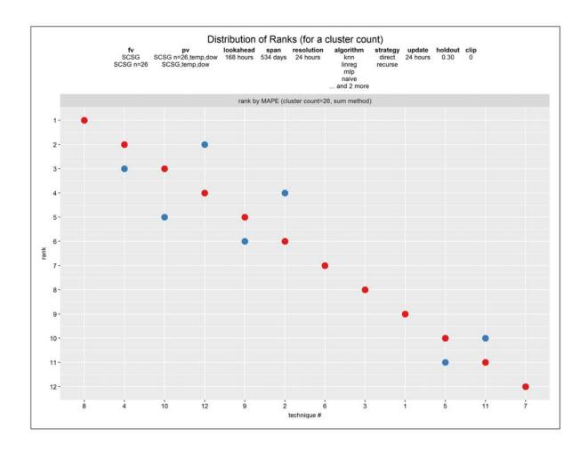
**Figure 6-49:** Effect of clustering – technique rank vs. technique at 26 clusters, Ireland, week-ahead forecasts. 12 techniques. Metric is MAPE. *Blue* is technique rank for a specific technique applied when grouping as 26 clusters. *Red* is technique rank for a specific technique applied without clustering.
