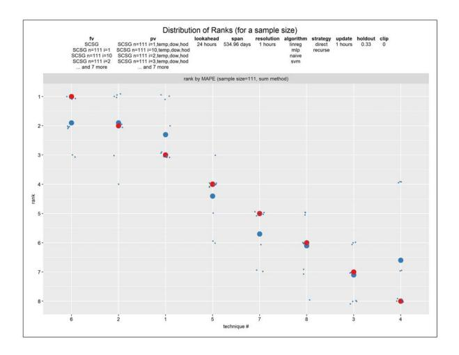
**Figure 6-46:** Effect of sampling — distribution of technique ranks across samples vs. technique at sample size 111, Australia, day-ahead forecasts. 8 techniques. Metric is MAPE. *Blue* is technique rank for a specific technique applied to 1 of 10 samples of size 111 out of 223. *Large blue* is mean technique rank for a specific technique applied to all 10 samples. *Large red* is technique rank for a specific technique applied to full population.
