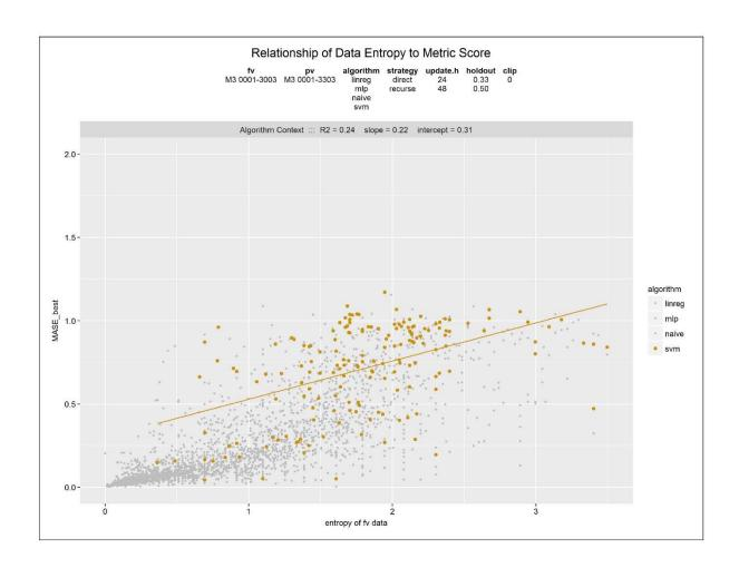
**Figure 3-9:** <u>Best metric score vs. entropy, support vector regression.</u> Data sources from the M3 Forecasting Competition. 3,003 data sources from x 32 techniques = 96,096 forecasts and evaluations. Evaluation by MASE score. Entropy values are arranged along the x-axis. *Gold* is best technique applied to one data source, filtered for support vector regression algorithm class.
