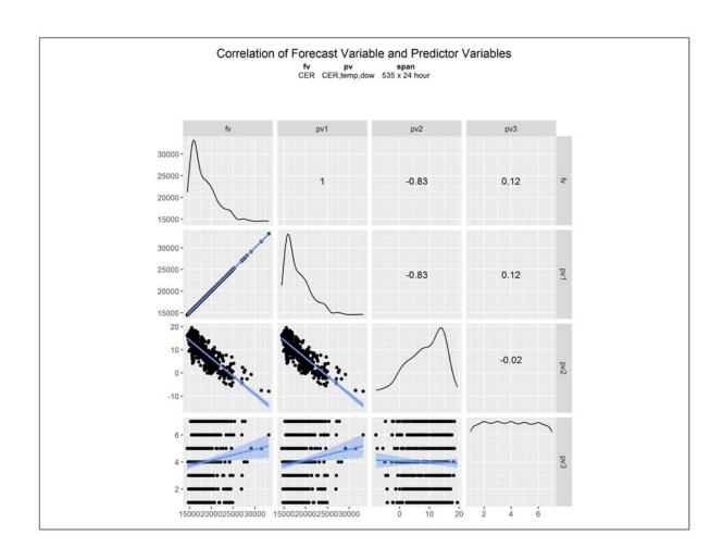
**Figure 4-4:** <u>Correlations of series, Ireland, for week-ahead forecasts.</u> Reference series is aggregated 782-household electricity usage. Predictor series are aggregate electricity usage, temperature, and day of week (integer coded).
