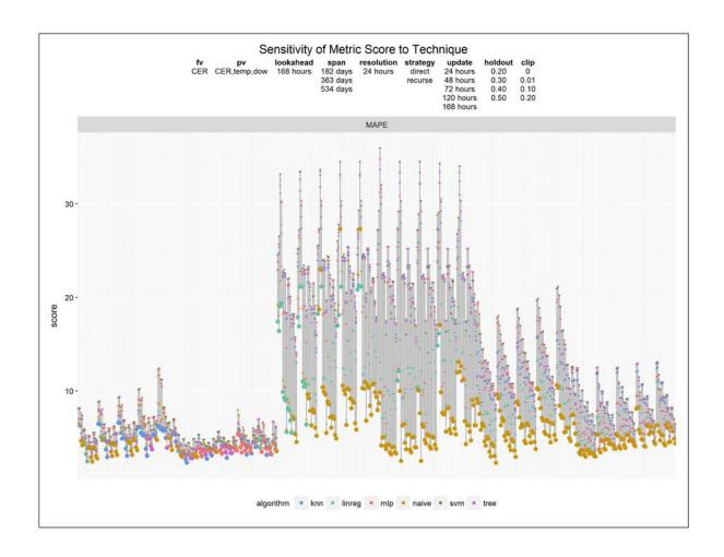
**Figure 4-12:** Distribution of metric scores across techniques, Ireland, week-ahead forecasts. 2,880 techniques and forecasts. Each vertical bar represents a family of techniques that differ from each other only by algorithm class. Distances along the vertical bars represent metric scores for specific techniques. Metric is MAPE. *Colors* are algorithm class. *Large point* is metric score of best technique within a family of techniques.
