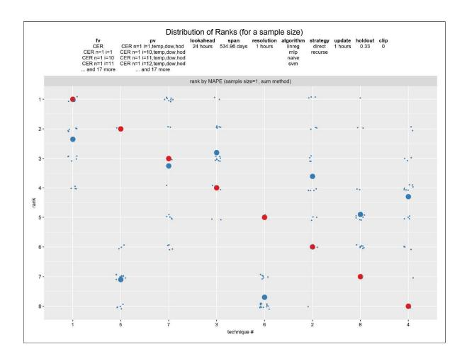
**Figure 5-16:** Effect of sampling – distribution of technique ranks across samples vs. technique at sample size 1, Ireland, day-ahead forecasts. 8 techniques. Metric is MAPE. *Blue* is technique rank for a specific technique applied to 1 of 20 samples of size 1 out of 782. *Large blue* is mean technique rank for a specific technique applied to all 20 samples. *Large red* is technique rank for a specific technique applied to full population.
