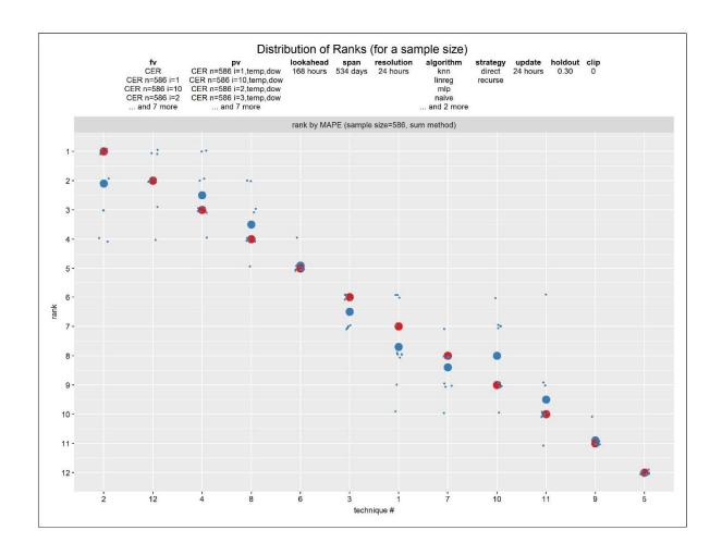
**Figure 5-15:** Effect of sampling – distribution of technique ranks across samples vs. technique at sample size 586, Ireland, week-ahead forecasts. 12 techniques. Metric is MAPE. *Blue* is technique rank for a specific technique applied to 1 of 10 samples of size 586 out of 782. *Large blue* is mean technique rank for a specific technique applied to all 10 samples. *Large red* is technique rank for a specific technique applied to full population.
