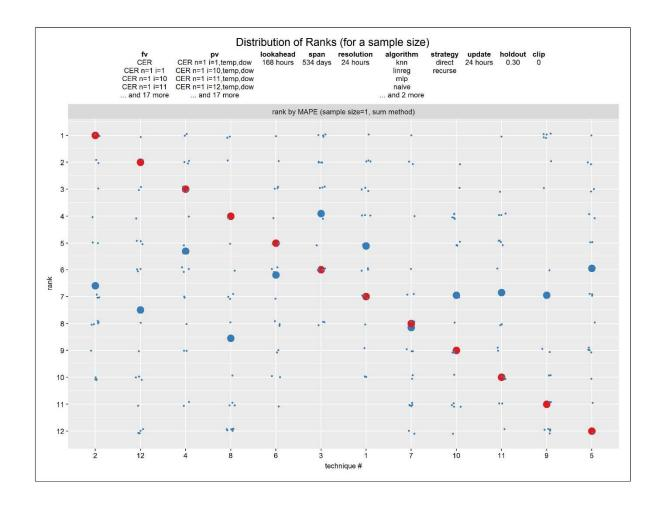
**Figure 5-10:** Effect of sampling – distribution of technique ranks across samples vs. technique at sample size 1, Ireland, week-ahead forecasts. 12 techniques. Metric is MAPE. *Blue* is technique rank for a specific technique applied to 1 of 20 samples of size 1 out of 782. *Large blue* is mean technique rank for a specific technique applied to all 20 samples. *Large red* is technique rank for a specific technique applied to full population.
