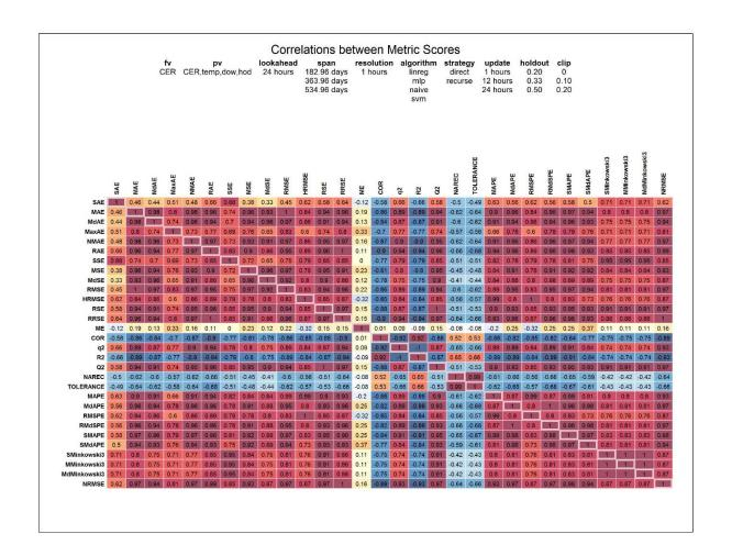
**Figure 4-19:** Correlations of scores per one metric-to-scores per another metric, across metric pairs, Ireland, day-ahead forecasts. 648 techniques and forecasts. For each cell, all techniques are scored per two metrics, and the sequence of scores per the first metric are correlated with the sequence of scores per the second metric. *Red* is positive correlation. *Blue* is negative correlation. *Dark* indicates strong absolute correlation. *Light* is weak absolute correlation.
