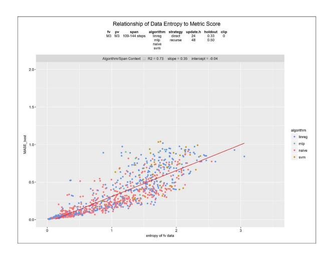
**Figure 3-13:** <u>Best metric score vs. entropy, long span.</u> Data sources of length 109-144 time steps from the M3 Forecasting Competition. 32 techniques. Evaluation by MASE score. Entropy values are arranged along the x-axis. *Colors* are algorithm class of best technique applied to one data source.
