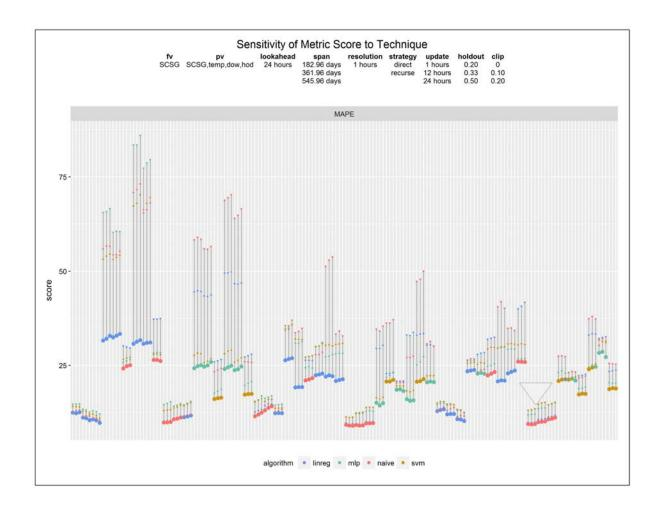
**Figure 6-9:** <u>Distribution of metric scores across techniques, Australia, day-ahead forecasts.</u> 648 techniques and forecasts. Each vertical bar represents a family of techniques that differ from each other only by algorithm class. Distances along the vertical bars represent metric scores for specific techniques. Metric is MAPE. *Colors* are algorithm class. *Large point* is metric score of best technique within a family of techniques.
