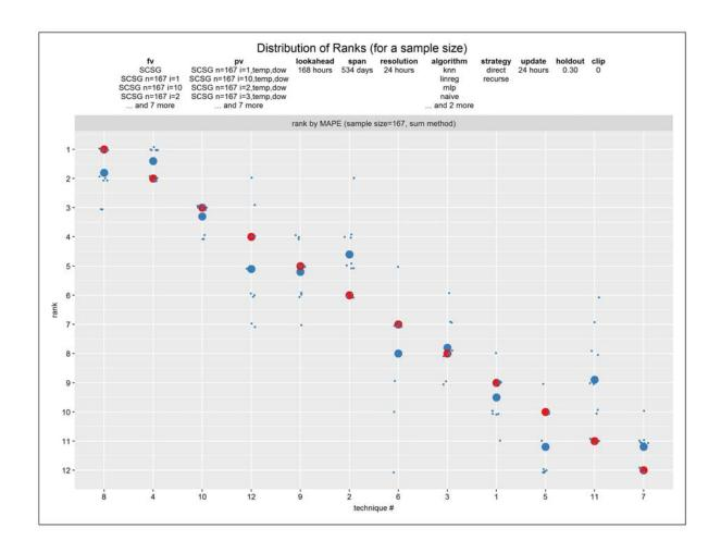
**Figure 6-44:** Effect of sampling – distribution of technique ranks across samples vs. technique at sample size 167, Australia, week-ahead forecasts. 12 techniques. Metric is MAPE. *Blue* is technique rank for a specific technique applied to 1 of 10 samples of size 167 out of 223. *Large blue* is mean technique rank for a specific technique applied to all 10 samples. *Large red* is technique rank for a specific technique applied to full population.
