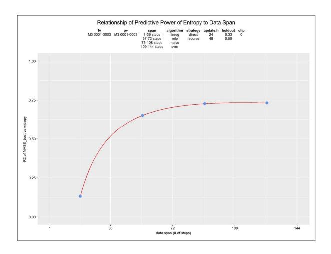
**Figure 3-14:** Correlation of metric score-to-entropy vs. data span. Data sources from the M3 Forecasting Competition. 3,003 data sources from x 32 techniques = 96,096 forecasts and evaluations. Evaluation by MASE score. Data spans are arranged along the x-axis.
