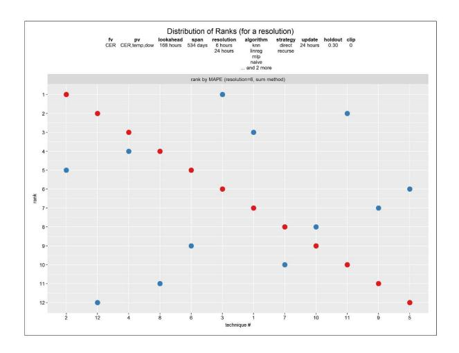
**Figure 5-29:** Effect of temporal magnification – technique rank vs. technique at short time step size, Ireland, week-ahead forecasts. 36 techniques (3 decision options for time step size, 12 combinations of other decision options). Metric is MAPE. *Blue* is technique rank for a specific technique applied at temporal magnification with 6-hour time step size. *Red* is technique rank for a specific technique applied without temporal magnification (baseline 24-hour time step size).
