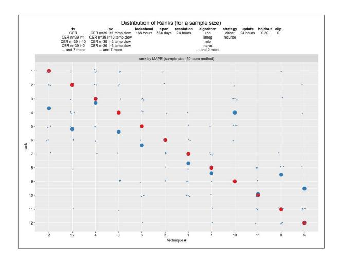
**Figure 5-11:** Effect of sampling – distribution of technique ranks across samples vs. technique at sample size 39, Ireland, week-ahead forecasts. 12 techniques. Metric is MAPE. *Blue* is technique rank for a specific technique applied to 1 of 10 samples of size 39 out of 782. *Large blue* is mean technique rank for a specific technique applied to all 10 samples. *Large red* is technique rank for a specific technique applied to full population.
