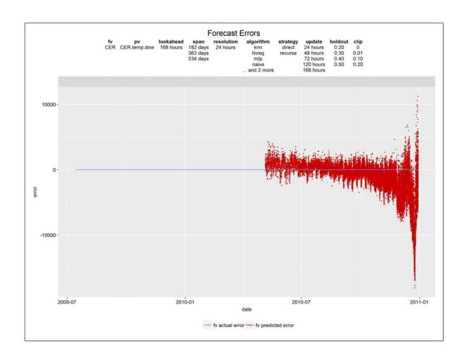
**Figure 4-7:** <u>Forecast error, Ireland, week-ahead forecasts.</u> 2,880 techniques and forecasts. *Blue* is reference series error (0). *Red* is overlay of forecast errors.
