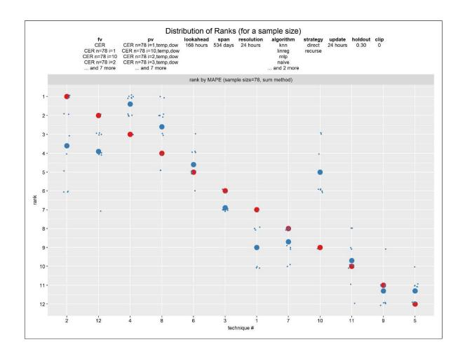
**Figure 5-12:** Effect of sampling – distribution of technique ranks across samples vs. technique at sample size 78, Ireland, week-ahead forecasts. 12 techniques. Metric is MAPE. *Blue* is technique rank for a specific technique applied to 1 of 10 samples of size 78 out of 782. *Large blue* is mean technique rank for a specific technique applied to all 10 samples. *Large red* is technique rank for a specific technique applied to full population.
