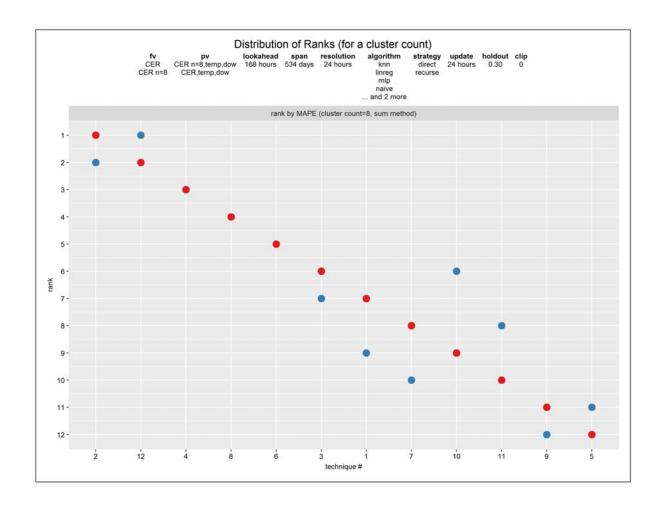
**Figure 5-24:** Effect of clustering – technique rank vs. technique at 8 clusters, Ireland, week-ahead forecasts. 12 techniques. Metric is MAPE. *Blue* is technique rank for a specific technique applied when grouping as 8 clusters. *Red* is technique rank for a specific technique applied without clustering.
