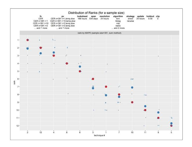
**Figure 5-14:** Effect of sampling – distribution of technique ranks across samples vs. technique at sample size 391, Ireland, week-ahead forecasts. 12 techniques. Metric is MAPE. *Blue* is technique rank for a specific technique applied to 1 of 10 samples of size 1391 out of 782. *Large blue* is mean technique rank for a specific technique applied to all 10 samples. *Large red* is technique rank for a specific technique applied to full population.
