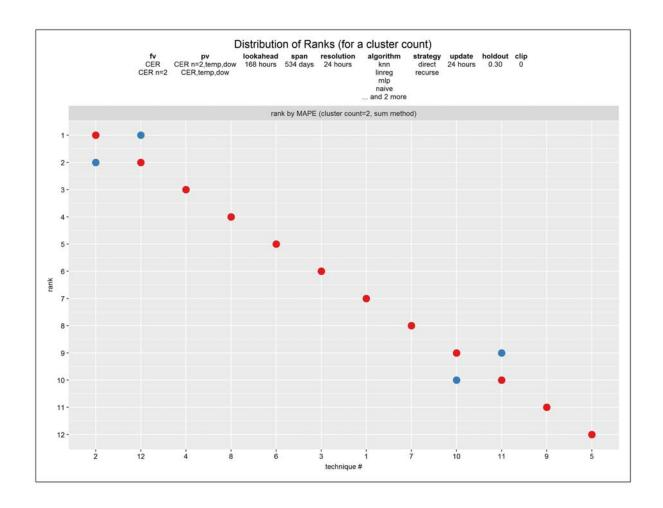
**Figure 5-22:** Effect of clustering – technique rank vs. technique at 2 clusters, Ireland, week-ahead forecasts. 12 techniques. Metric is MAPE. *Blue* is technique rank for a specific technique applied when grouping as 2 clusters. *Red* is technique rank for a specific technique applied without clustering.
