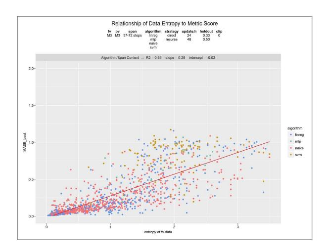
**Figure 3-11:** <u>Best metric score vs. entropy, medium span.</u> Data sources of length 37-72 time steps from the M3 Forecasting Competition. 32 techniques. Evaluation by MASE score. Entropy values are arranged along the x-axis. *Colors* are algorithm class of best technique applied to one data source.
