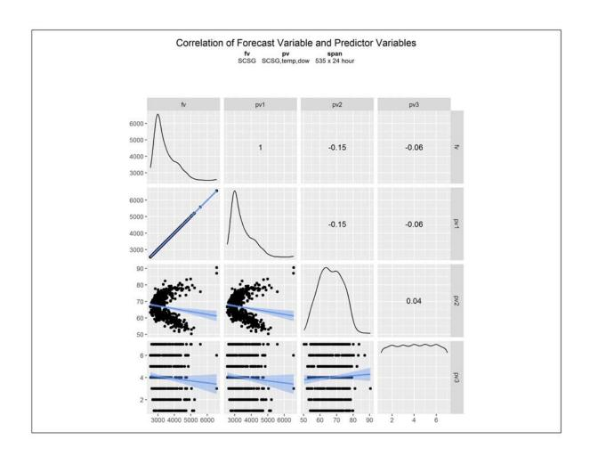
**Figure 6-4:** Correlations of series, Australia, for week-ahead forecasts. Reference series is aggregated 223-household electricity usage. Predictor series are aggregate electricity usage, temperature, and day of week (integer coded).
