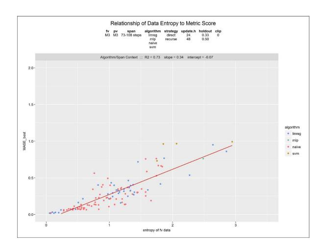
**Figure 3-12:** Best metric score vs. entropy, medium-long span. Data sources of length 73-108 time steps from the M3 Forecasting Competition. 32 techniques. Evaluation by MASE score. Entropy values are arranged along the x-axis. *Colors* are algorithm class of best technique applied to one data source.
