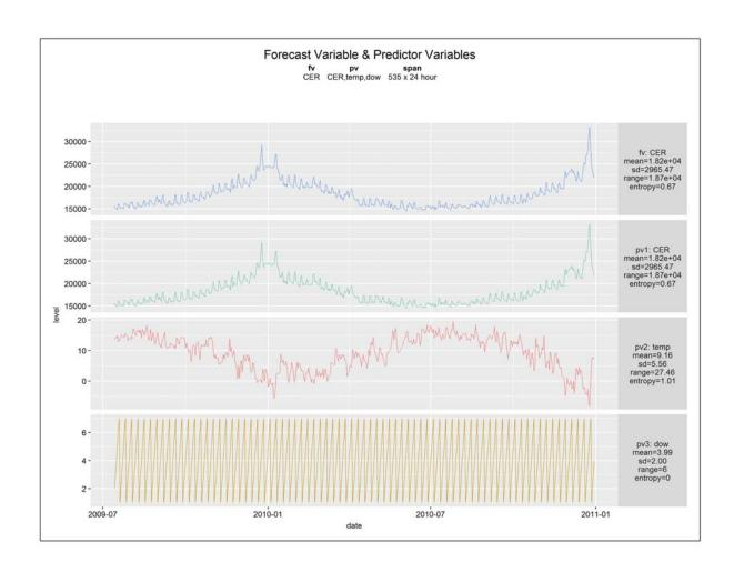
**Figure 4-3:** Reference and predictor series, Ireland, for week-ahead forecasts. Reference series is aggregated 782-household electricity usage. Predictor series are aggregate electricity usage, temperature, and day of week (integer coded).
