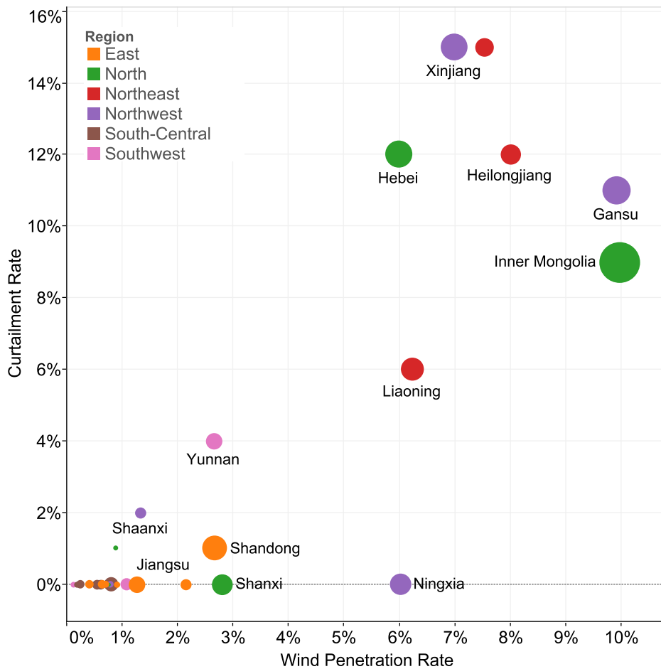
Figure 3.3: 2014 wind curtailment rates in various provinces (the circle areas are proportional to the installed capacity). Provinces with high wind penetration rates tend to have high curtailment rates as well. Plot produced by authors using data from CWEA (2015) for wind installed capacity, NEA (2015a) for electricity generated by wind, and NBS (2014) for total electricity generation.
