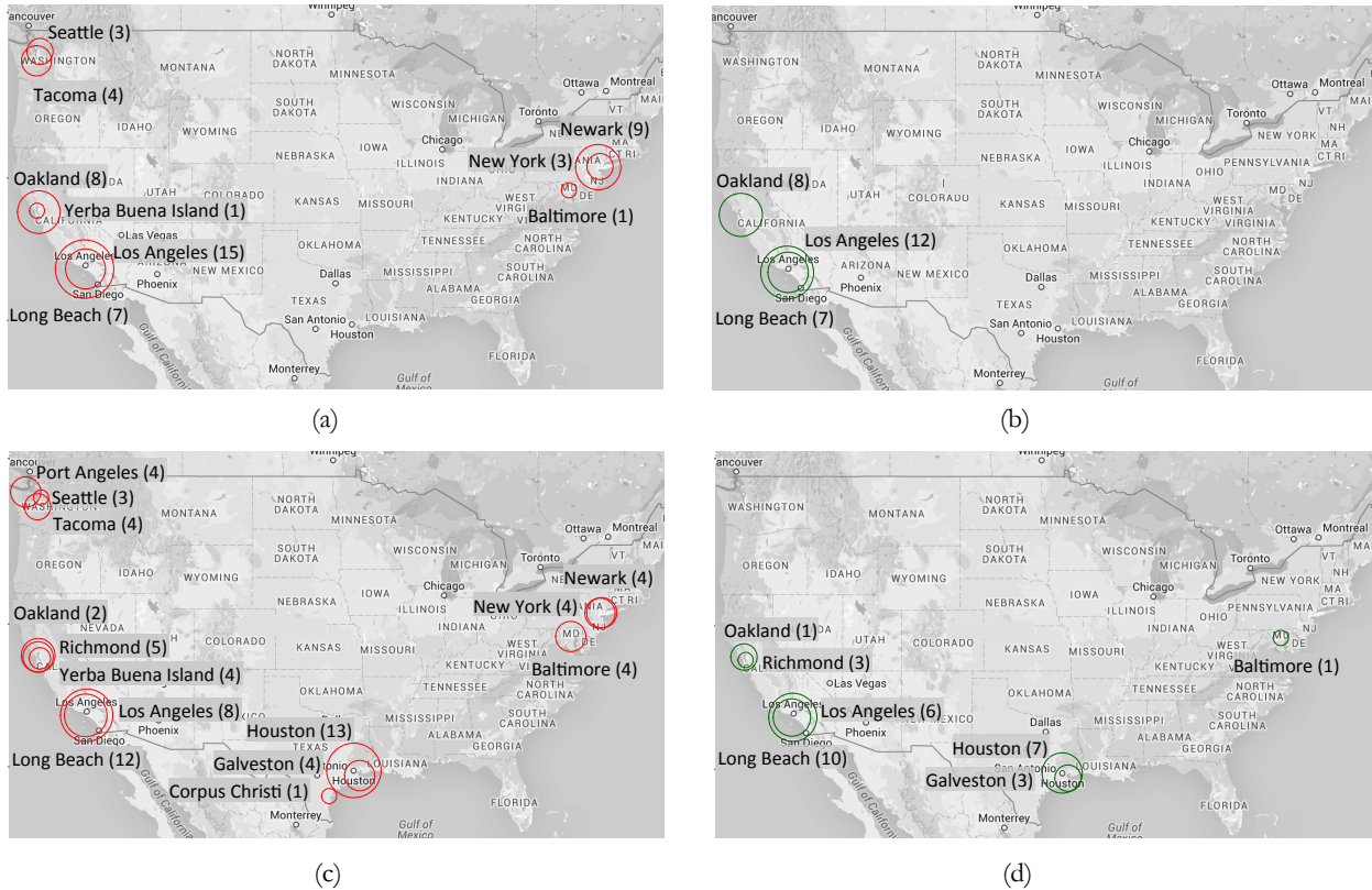
Figure 5.16: Geographical distribution of berths that it is optimal to retrofit in order to maximize the total net benefit for (a) container and bulk cargo vessels assuming social costs of pollution derived from EASIUR, (b) container and bulk cargo vessels assuming APEEP, (c) tankers and vehicle carriers assuming EASIUR, and (d) tankers and vehicle carriers assuming APEEP. The number in the bracket indicates the number of berths that ought to be retrofit in the optimal solution. For container vessels, the optimal solution based on APEEP is to simply concentrate on California, whereas the optimal solution in EASIUR involves retrofitting ports in the Pacific Northwest as well as in the northeast United States. For tankers and vehicle carriers, assuming the social costs in APEEP again produces a solution that is dominated by California ports, with some use of shore power in the Gulf of Mexico. Using EASIUR produces a solution in which a large number of ports across the country ought to be retrofit.
