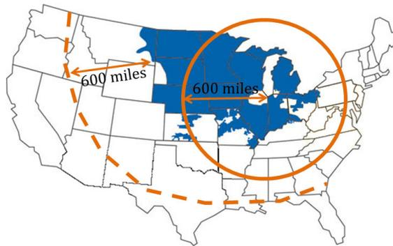
Figure 3.2 Limit of AC transmission distance considered in the analysis to any Midwest ISO node (dashed line) and to a major load center (solid line)
