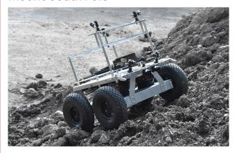
MoonRanger, a small robotic rover being developed by Carnegie Mellon University and its spinoff <u>Astrobotic</u>, has completed its preliminary design review in preparation for a 2022 mission to search for signs of water at the moon's south pole.
