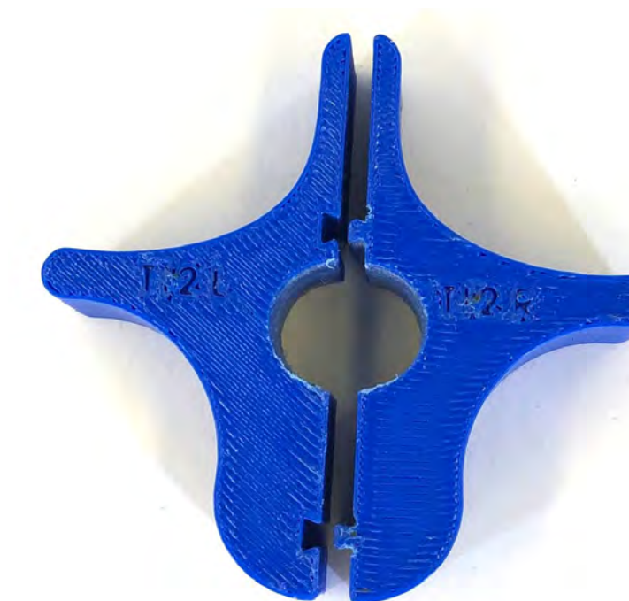
Figure 6. Vertebra with Dovetail Connection
