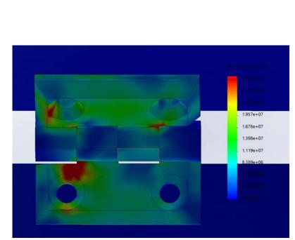
Prototype #3 FEA Analysis with Von Mises Stress (N/m^2) under loading conditions of average male body weight [3]
