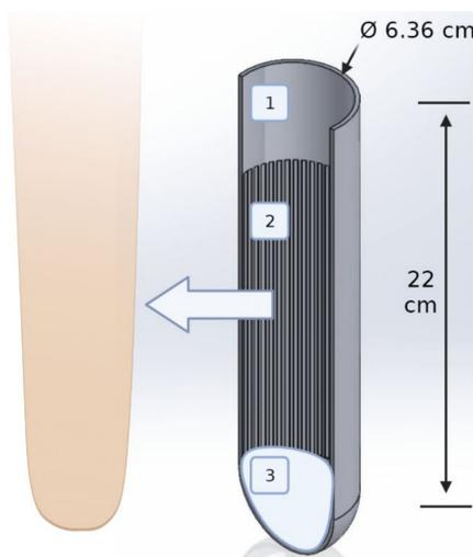
Fig. 1: CAD cross-section representation of a silicone lower limb prosthetic liner with interior channels to wick sweat downwards towards a removable absorbent pad.
