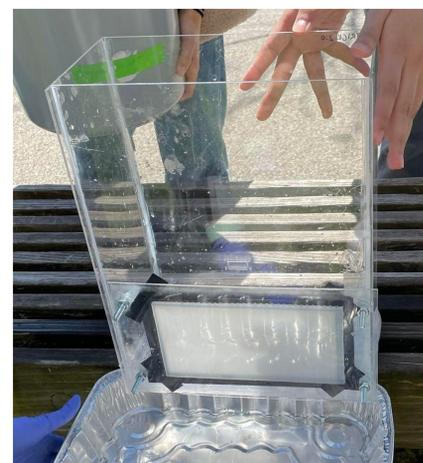
Fig. 4 Front view of experimental setup with liner pressed against membrane-based reservoir flow panel
