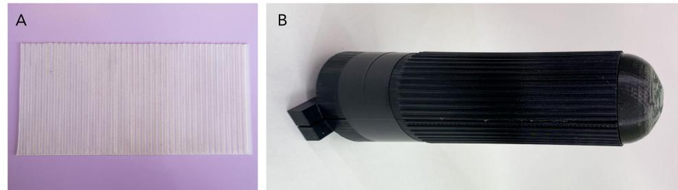
Fig. 2: A. Flat silicone sheet fabricated in a 3D printed mold with channels. B. Final 3D printed mold for liquid silicone. This inner mold rests in an outer cylindrical shell to create a single silicone piece with both channeled and non-channeled regions.
