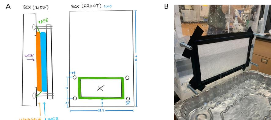
Fig. 3: A. Side and front view schematic of the membrane based reservoir flow panel. B. water flowing through a double layered 10 micron membrane
