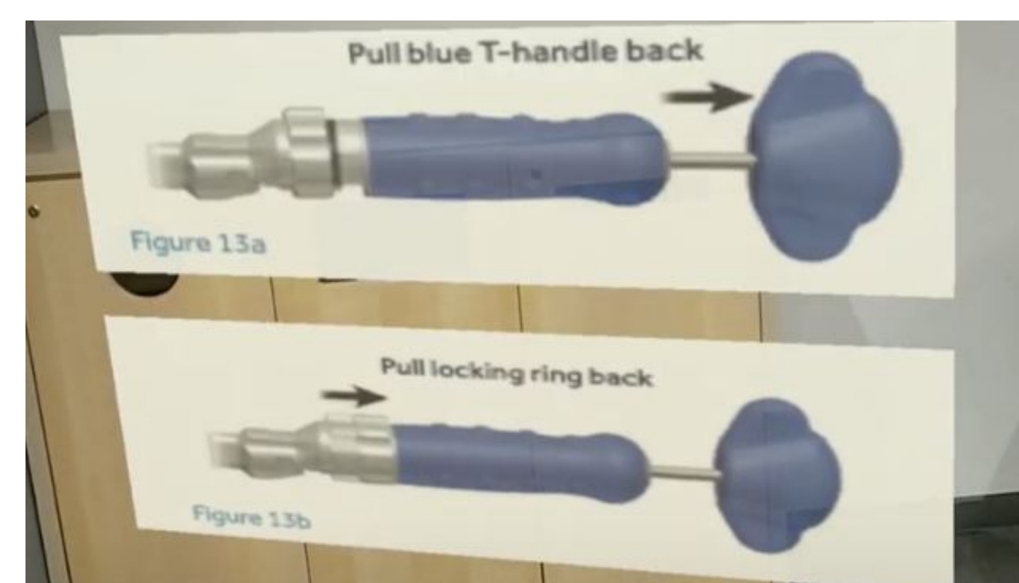
Figure 4: Step-by-step instructions for attaching centerpiece to inserter which user can scroll through with their hands
