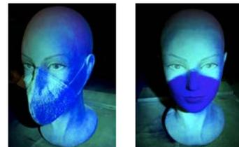
The mask and seal were effective at preventing particle penetration as shown by the absence of spray paint beneath the mask area
