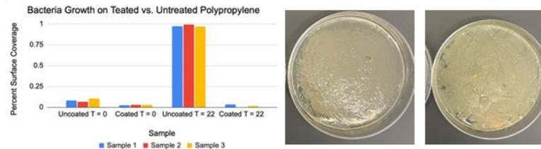
The antibacterial activity from four independent test groups, T-0 hrs and T-22 hrs for both coated and uncoated samples, show that the salt coating on the polypropylene fabric effectively reduces E.coli growth and surface coverage
