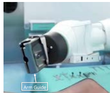
Figure 3: A close up of the arm guide attached to the robotic system with no plastic drape intermediary 5
