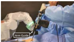
Figure 2: Surgeons using the Mazor X Stealth Edition. The surgical tools are guided through the arm guide to the patient. 4
