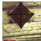
Figure 6: Microhardness indentation of PETG
