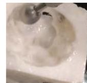
Figure 7: Drilling through temporal bone model with otologic drill and diamond burr
