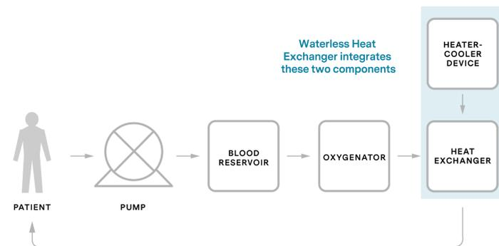
FIG 1. Overall Schematic of how an HCD works in conjunction with a CPB and how our device integrates with a CPB.
