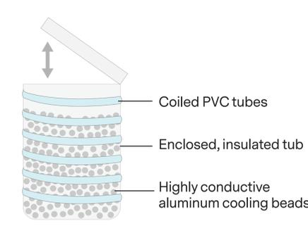
FIG 3. Cooling Unit Diagram.
