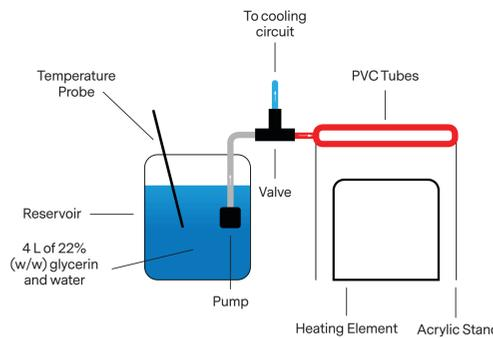
FIG 2. Heating Circuit Diagram.
