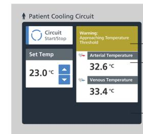
FIG 7. Control panel with warning status.
