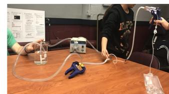
^ Figure 8: Assembled Blood Flow Circuit
