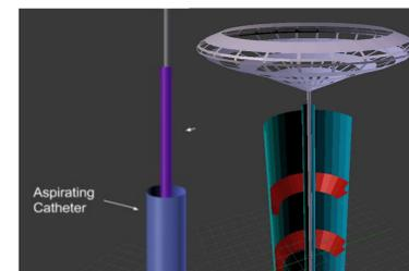
^ Figure 3: CAD Model of Aspiration Sheath and Filter
