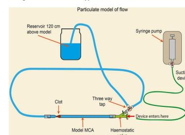
^ Figure 6: Schematic of blood flow circuit
