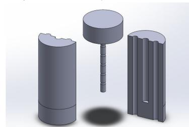
^ Figure 4: Catheter Mold Prototype in SolidWorks
