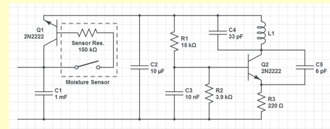
Figure 3. Schematic depicting the layout implemented in the sensor circuit.
