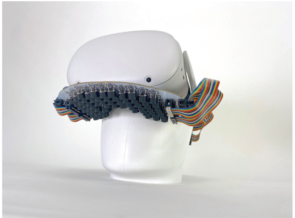
VR headset with mouth haptics add-on. Future Interfaces Group
