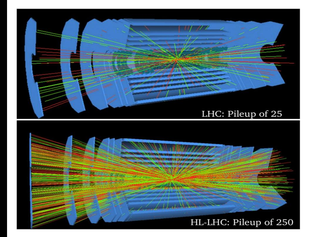
The ability to distinguish particles produced in the primary interaction from the spurious particles produced in the secondary interactions is key to the CMS physics program.
