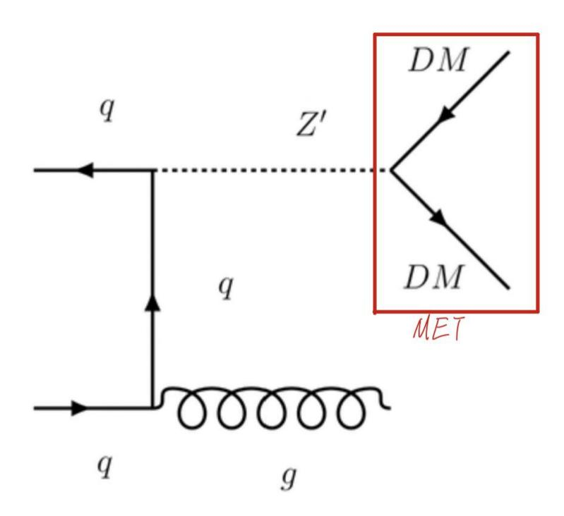
Once produced, since they are weakly interacting, DM particles would not interact with the CMS detector. However, they can manifest themselves as an imbalance in the transverse momentum, if produced in association with visible particles. At CMS, an entire program has been built on searches for DM in events with large missing transverse momentum (MET).
