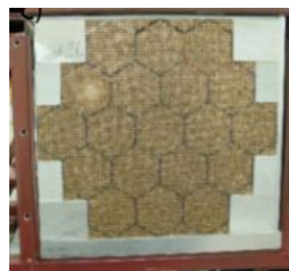
Figure 2: Hexagonal transverse towers in the original DREAM detector
