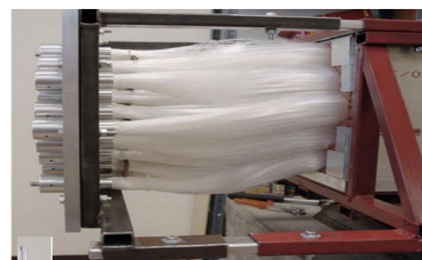
Figure 1: Bundles of scintillating and plastic fibers in the original DREAM prototype
