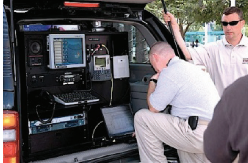
Mobile Communicator Vehicle (MC2): NIMS Type IV (with satellite, VoIP)
