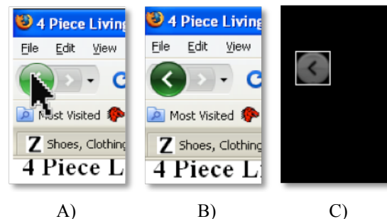
Figure 3: Selected Target found by calculating the difference between images taken during a locator button's press and release events. A) The user is pressing on the "Back" button in Firefox (the cursor here is for illustration only and not captured in our data). B) The image captured after the user releases the button. C) After subtracting A from B, the resulting difference is the correct target (shown with a bounding box).
