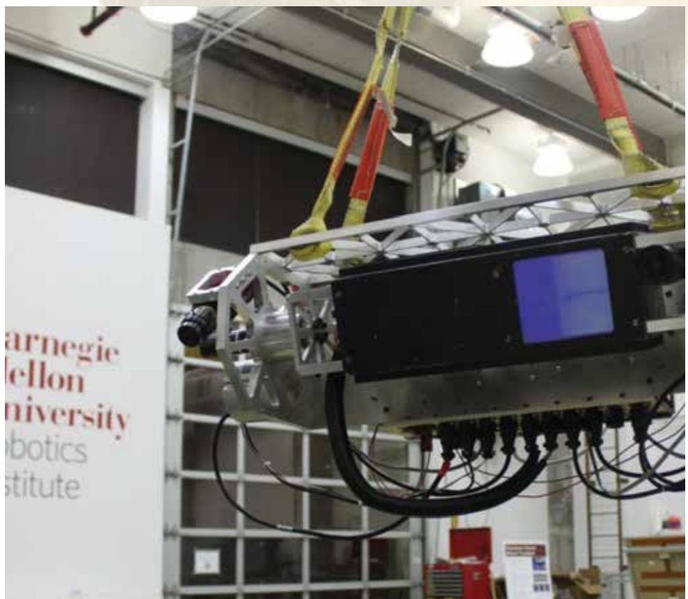
THE SENSOR PACKAGE USES COMPUTER VISION TO BUILD A 3-D MODEL OF THE LARGE PITS IN THE SURFACE OF THE MOON AND MARS.
