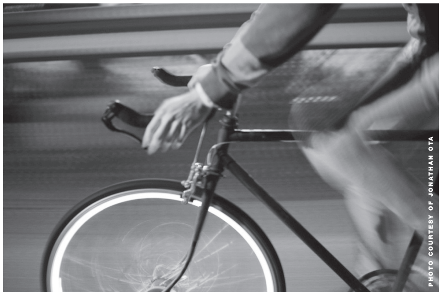
JONATHAN OTA AND ETHAN FRIER INSERTED LED LIGHTS INTO THE RIMS OF THEIR BICYCLE WHEELS TO INCREASE THEIR VISIBILITY IN TRAFFIC AND AMONG PEDESTRIANS.
