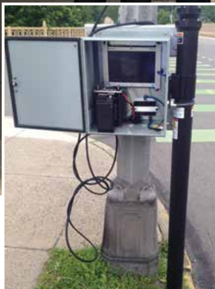
BERNARDO PIRES (SECOND FROM RIGHT) AND HIS TEAM HAVE BEEN WORKING TO COLLECT DATA ON HOW MUCH BIKE LANES ARE ACTUALLY BEING USED. TEAM MEMBERS ARE (L-R) MEHMET KOCAMAZ, JOHN KOZAR AND JIAN GONG. AT LEFT: A PORTABLE, COMPUTER-VISION DEVICE THEY'VE BUILT RECORDS AND COUNTS INDIVIDUAL USERS.
