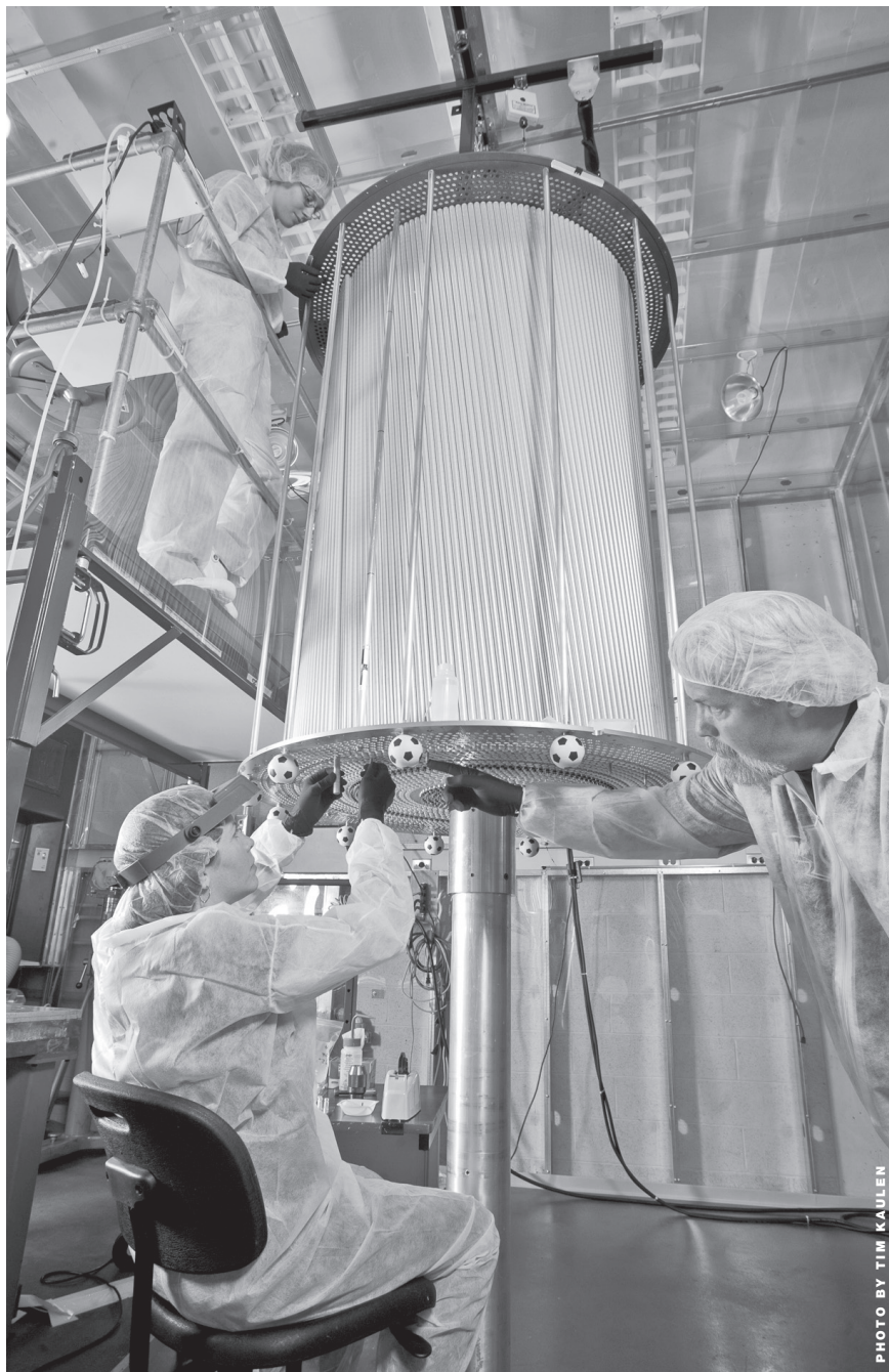
TEAM MEMBERS, CLOCKWISE FROM TOP, MADDISON BRUMBAUGH, A JUNIOR IN APPLIED PHYSICS AND INTERNATIONAL RELATIONS AND POLITICS, AND GARY WILKIN AND AMY WOODHALL, PHYSICS TECHNICIANS, WORK ON THREADING WIRE THROUGH EACH TUBE IN A REACTION CHAMBER ON A PARTICLE DETECTOR BEING BUILT AT CARNEGIE MELLON.
