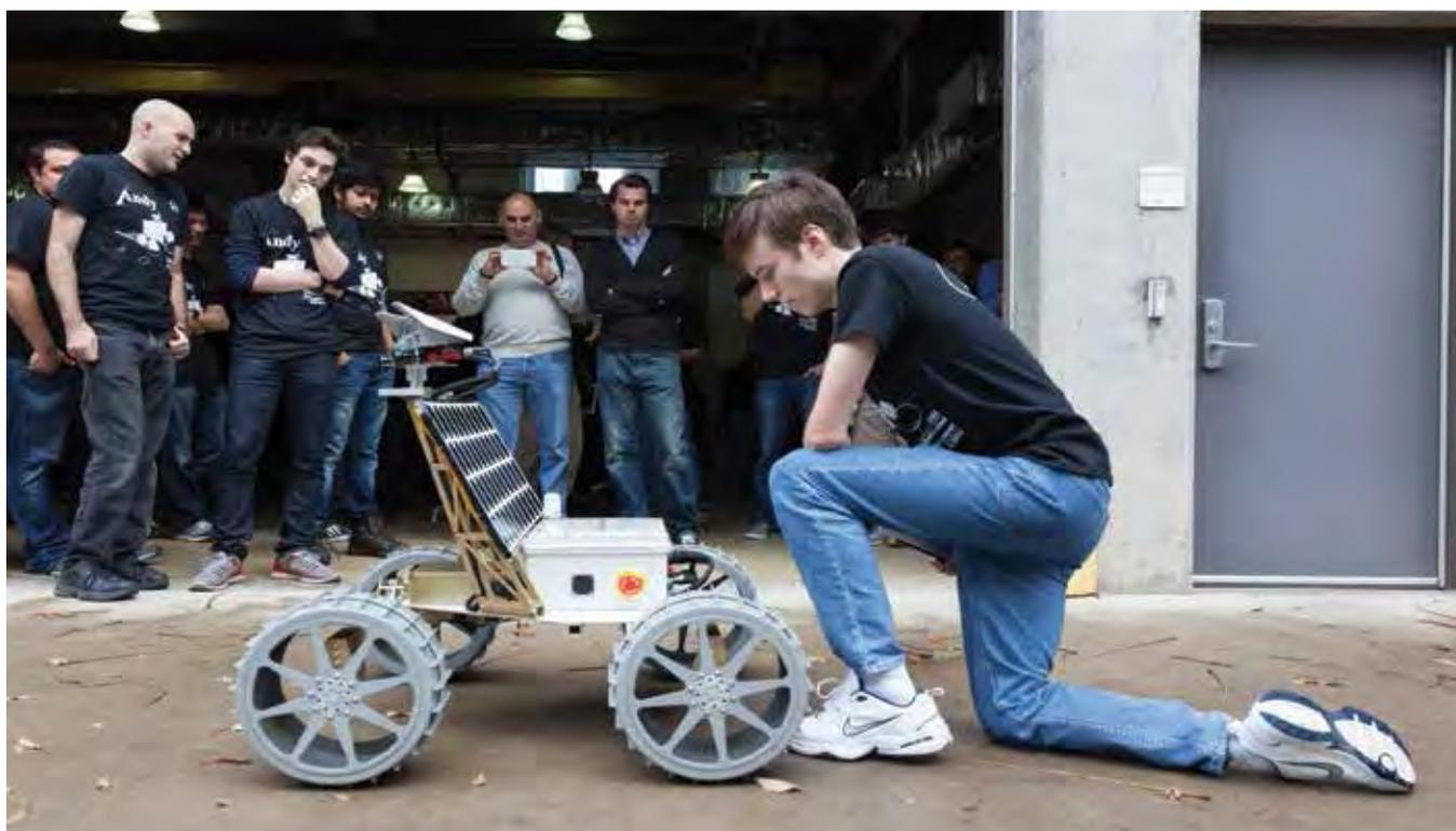
JUNIOR COMPUTER SCIENCE MAJOR JOHN MANN (PICTURED ABOVE) DEVELOPED SOFTWARE FOR ANDY, A FOUR-WHEELED ROBOT DESIGNED TO SCRAMBLE UP STEEP SLOPES AND SURVIVE THE TEMPERATURE SWINGS AND HIGH RADIATION ENCOUNTERED WHILE EXPLORING THE MOON'S PITS, CAVES AND POLAR ICE.
