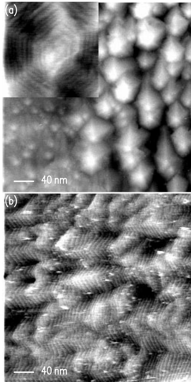
Figure 4 (a) AFM image of 200 nm thick film of GaN grown at 550°C. The 0.5 $\mu\text{m}$  $\times$ 0.5 $\mu\text{m}$  inset shows a close-up of a spiral growth mound. Greyscales of the large image and the inset are 83 Å and 20 Å respectively. (b) AFM image of a 200nm thick GaN film grown at 650°C. Greyscale for this image is 15.9 Å.
