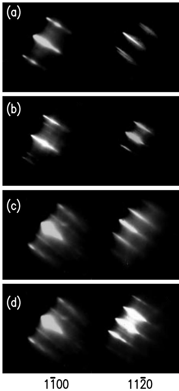
Figure 1 RHEED patterns in the  $[1\bar{1}00]$  and  $[11\bar{2}0]$  directions for GaN on 6H-SiC (0001) shown in order of decreasing surface Ga content (a) pseudo  $1\times 1$ , (b)  $4\times 6$ , (c)  $2\times 1$  and (d)  $2\times 2$ .
